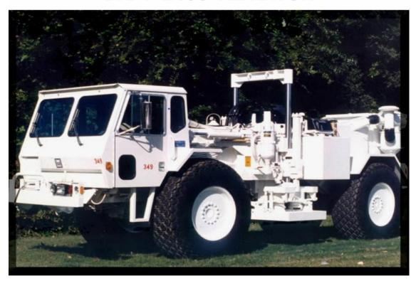
The 'birdwagen' MARK IV off-road carrier with the Failing Y-2400 vibrator. This is an advanced seismic source production system designed for high quality and high production geophysical prospecting. The 48,000 pound output vibrator offers broad band output and a high signal to noise ratio for the deepest surveys.
