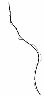
**Figure 2**. South Porcupine high-resolution and regional line (101A and 101, respectively). The fine line is the surface shotpoint line (i.e., the road traverse line). The heavy line is the Common Depth Point (CDP) line, which follows the mid point between the sources and the receivers. The CDP, developed in the processing, has the effect of smoothing out the sharp turns in the line, and more closely represents the locations of features in the seismic section.
