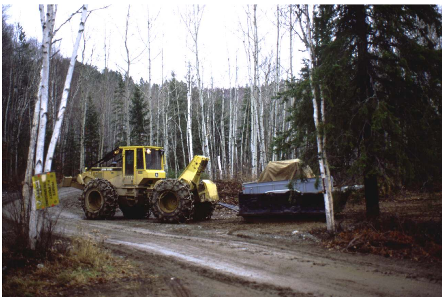
Figure 15.4: Image showing how the winch and trailer was transported from N-40 to N-43. A sloop designed for moving drilling rods was used to carry the DSI equipment.
