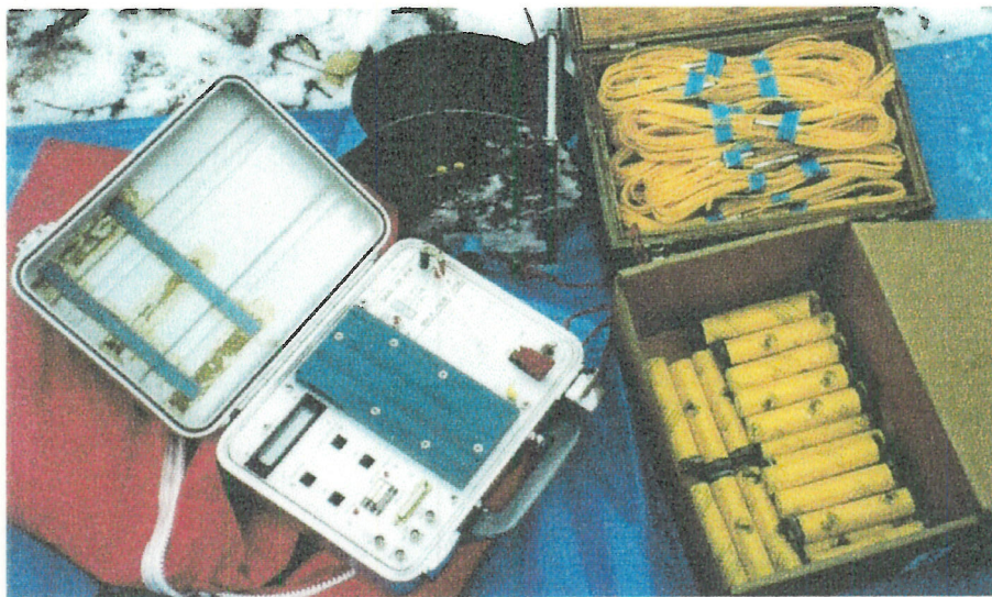
Figure 6: Blasters equipment at Norman West including a blasting box, seismic caps, penth-lite boosters and firing line.
