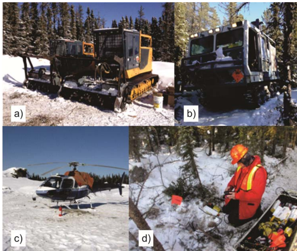
Figure 3. a) Mulchers used to cut lines for the active source 3D survey b) Shot hole drilling truck, c) Survey helicopter d). Interferometry installation.
