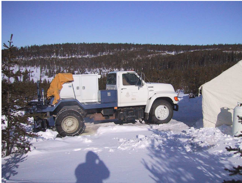
Figure 1: Vibrator during the data acquisition in borehole MC218, McArthur River Mine (Saskatchewan). Photo by Erick Adam, February 2001.
