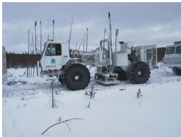
Figure 3 - Kinetex Vibroseis truck used for regional and high-resolution profiling.
