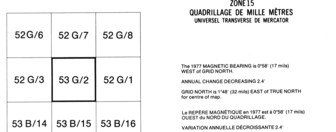
The 1977 MAGNETIC BEARING is 058° (17 mils) WEST of GRID NORTH.
