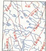
The declination of the compass needle at any place along a red line is the declination given on that red line. At other places the declination is between those given on the neighbouring red lines; that at the place marked A, the declination is between N. 39° E. and N. 39° E. The westerly declinations of the compass needle are decreasing 12 minutes annually.
