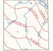
The declination of the compass needle at any place along a red line is the declination given on that red line. At other places the declination is between those given on the neighbouring red lines; that at the place marked 'A', the declination is between 11° 15' E and 11° 30' E. The easterly declinations of the compass needle are decreasing 6.6 minutes annually.
