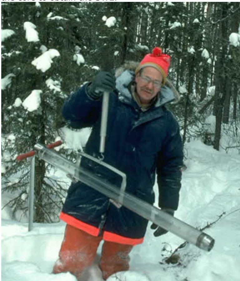
Figure 3. Scientist Using a Weighing Snow Sampler. The spring balance gives a direct reading of water equivalent in millimetres. The sample is bagged and subsequently weighed indoors when wind makes weighing difficult.
