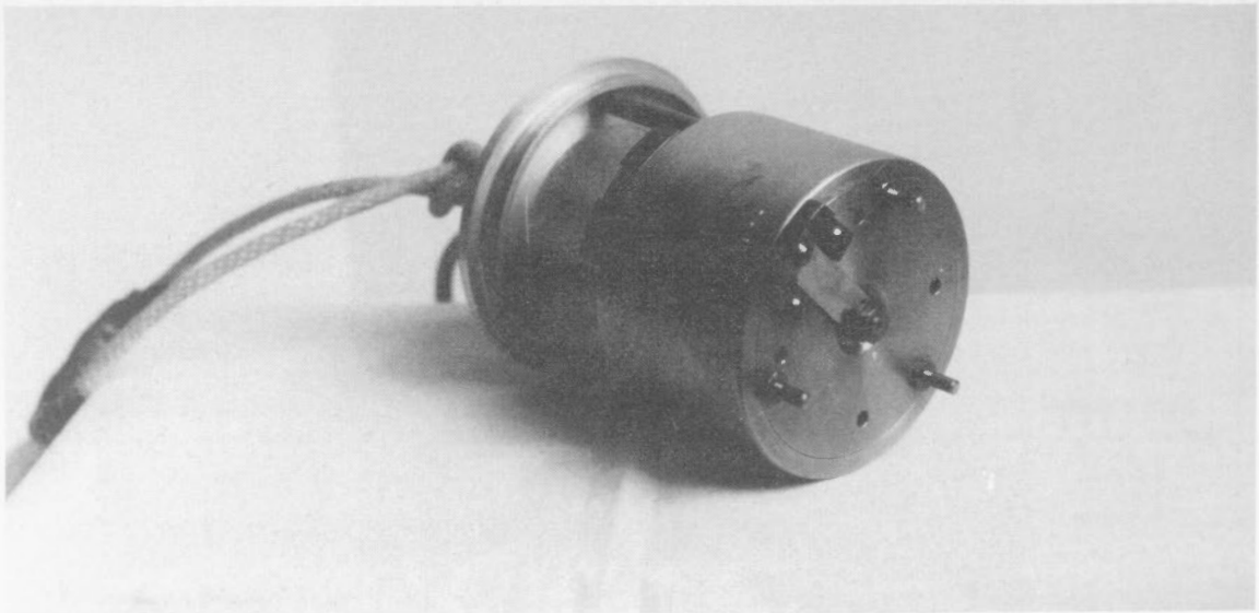
Fig. 18 Interior Heiland Geophone, Mine Seismograph.
