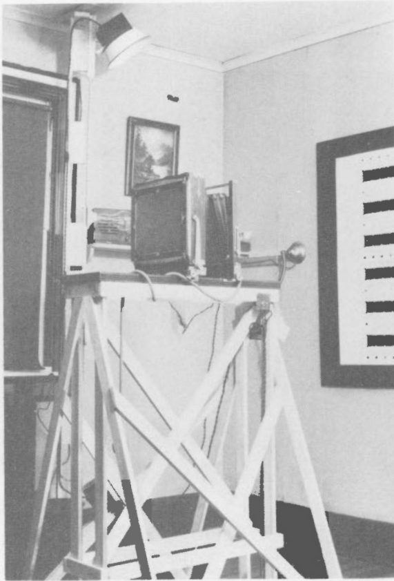
Fig. 75 Fixed Camera Placement for Record Photography.
