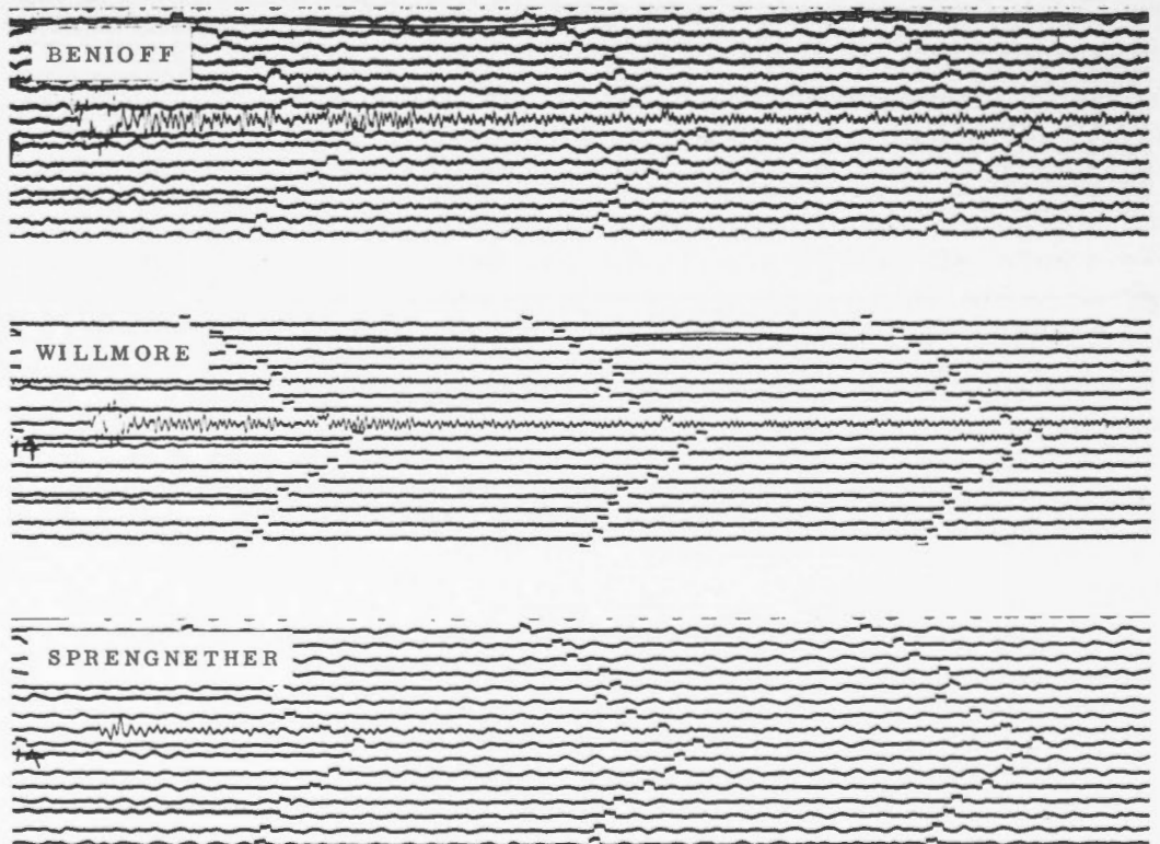
Figure 13. Short-period vertical seismograms from earthquake in Outer Mongo- lia, December 4, 1957, \Delta = 59^\circ .
