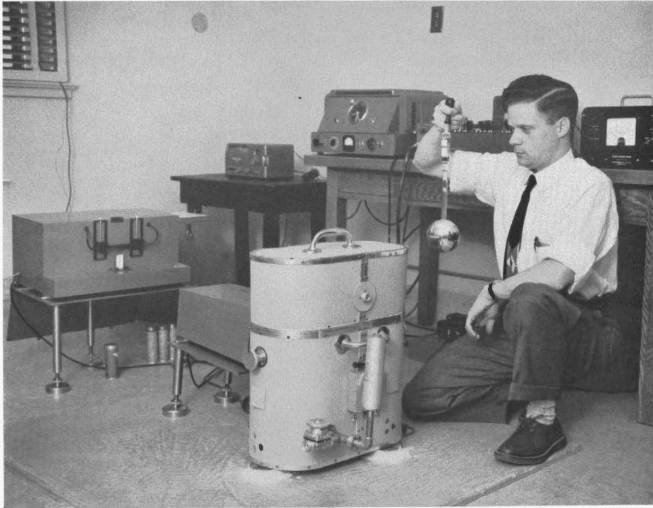
The pendulum apparatus set up on the new pendulum pier in the Geophysical Laboratory of the Dominion Observatory. The author is holding one of the gilded bronze pendulums.
