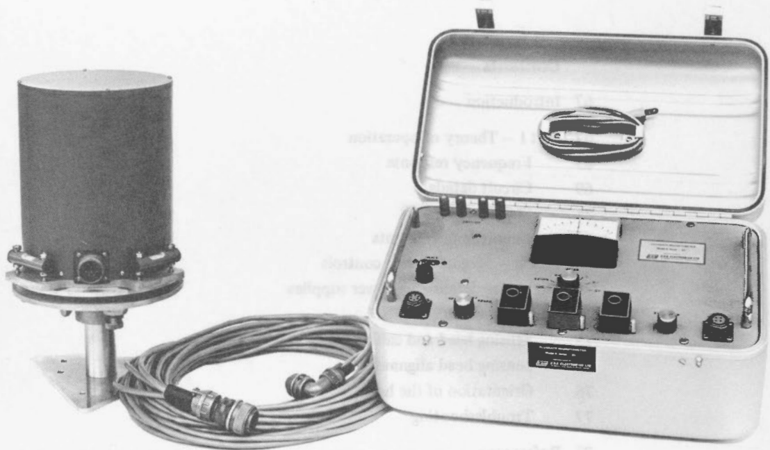
Figure 1. The solid-state, 3 component magnetometer.
