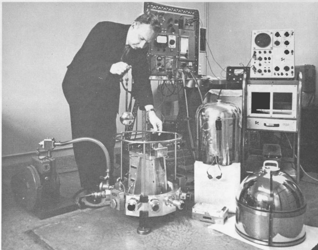
Figure 3. View of the pendulum apparatus, with the bell jar and oven-cover removed, showing the radiation shield.
