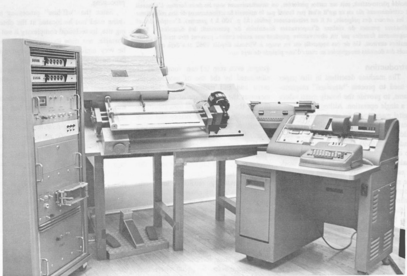
Figure 1. Overall view of magnetogram reader with keypunch and printer, shown set up for left-handed operator.
