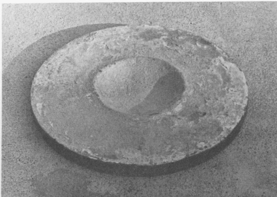
FIGURE 1(a). Model crater in the form of a brass casting. Diameter of crater rim 12.7 cm. Depth of crater (rim to floor) 1.7 cm. Over-all diameter of casting 29.7 cm. The surface of the model has been roughened by the process of chemical deposition (C.S. Beals).
