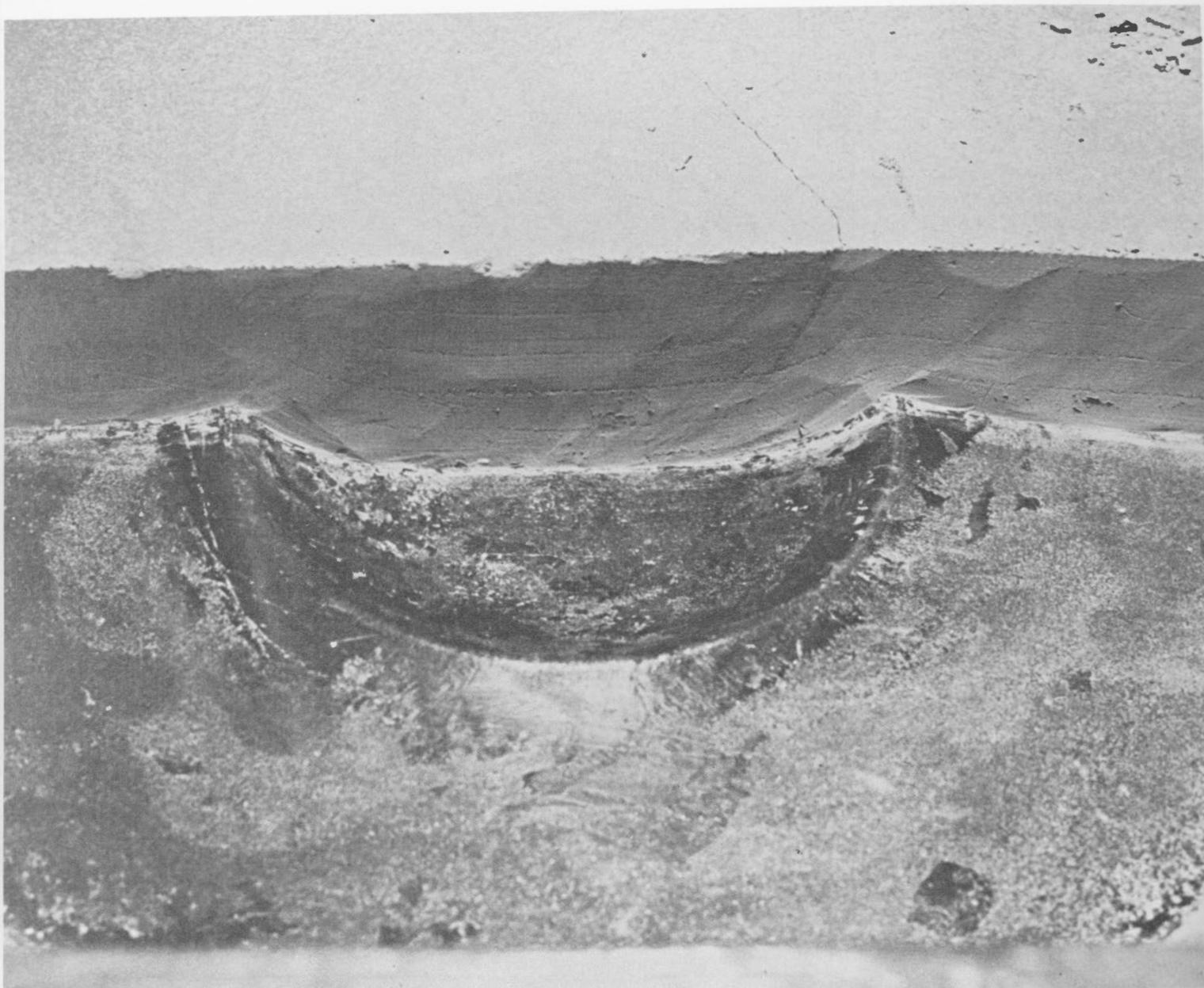
FIGURE 3. Section of sedimentary covering of model crater. In the foreground appears one half of the brass crater model from which the sedimentary covering has been removed. In the background the five main layers of sediment are clearly seen with faint indications of nine 'varves' in each layer.
