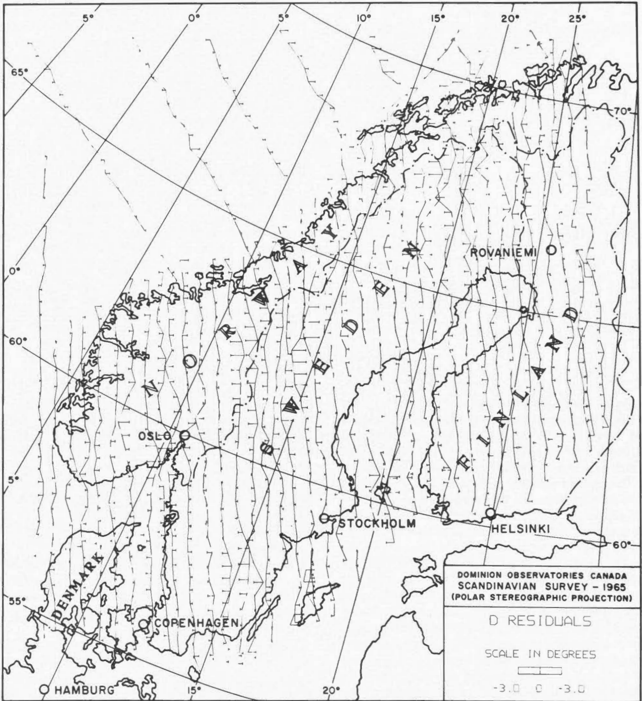
FIGURE 12. Nordic survey Declination profiles of the 5-minute average residuals.
