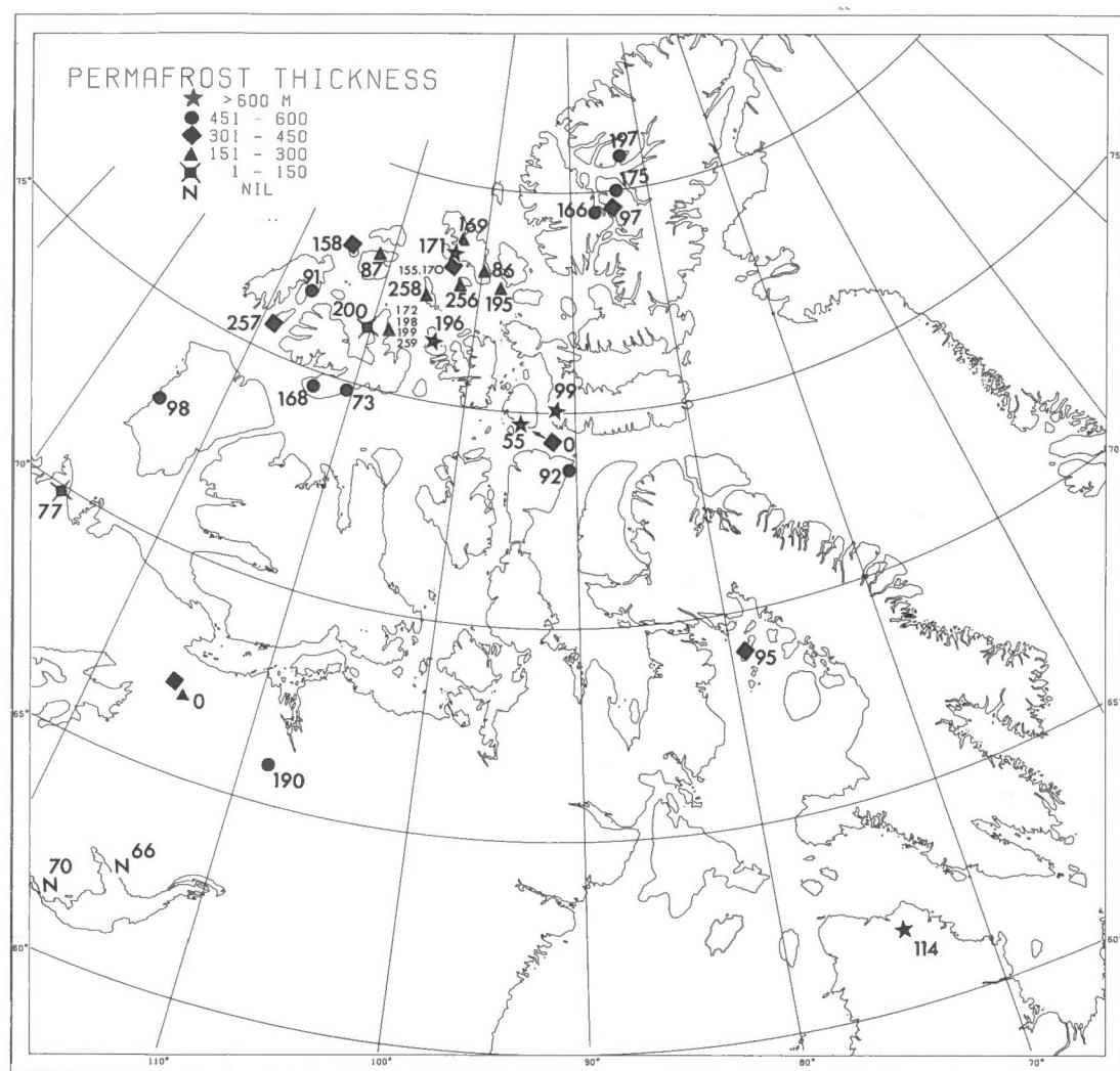
Figure 1. Site locations and permafrost thicknesses for Northern Canada (excluding the Mackenzie Valley and Delta). The symbols represent permafrost thicknesses in metres, and the numerals are Earth Physics Branch file numbers as used in Tables 1 and 2.
