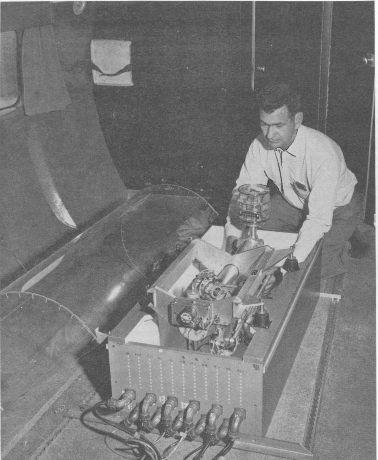
Figure 2. The gyro-stabilized platform and fluxgate sensor assembly.
