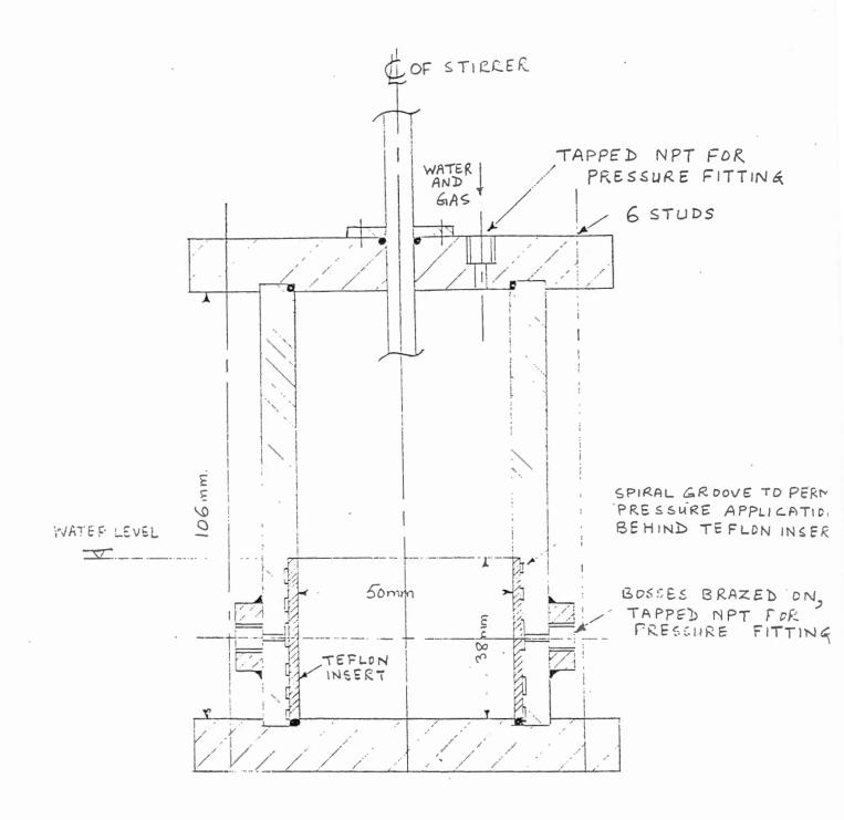
FIGURE 1. LOW PRESSURE (IMPA) CELL FOR FORMING HYDRATE SPECIMENS.
