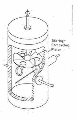
FIGURE 2. STIRRER WITH STIRRING--COMPACTING PLATEN
