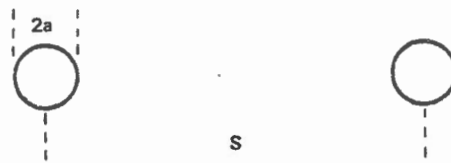
PARALLEL TRANSMISSION LINE
