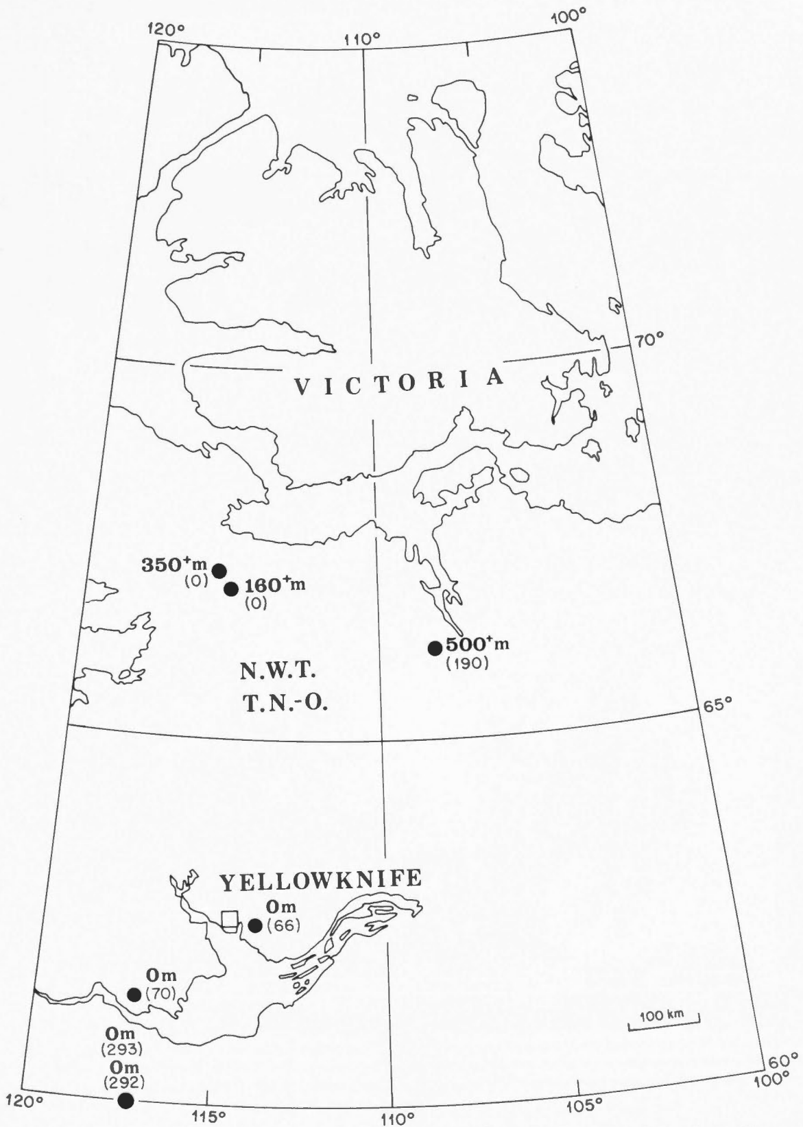
Figure 4. Site locations and permafrost thicknesses (metres) in the Western Arctic. The numerals in brackets are Earth Physics Branch file numbers.
