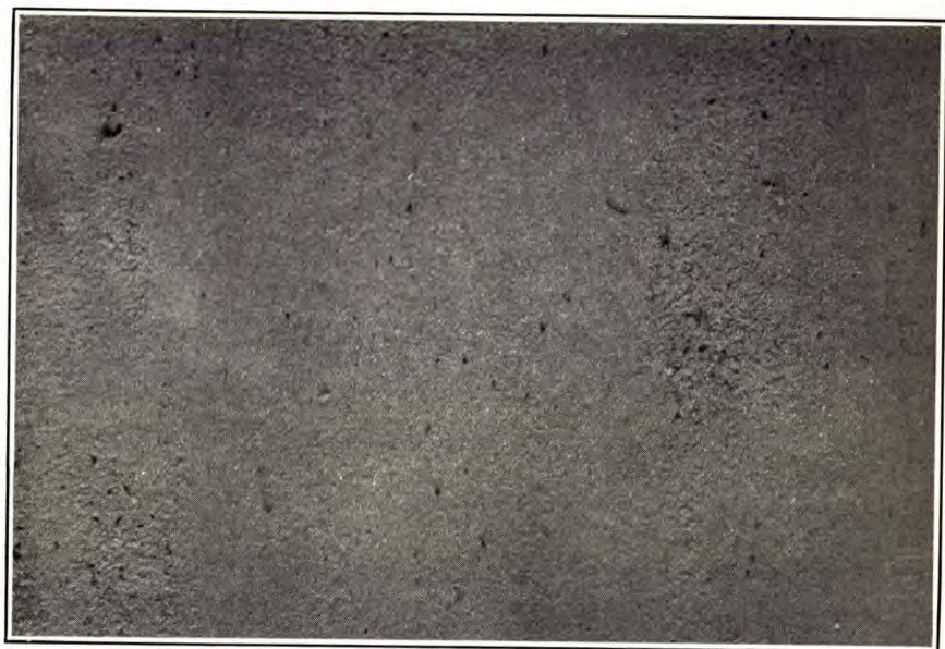
A. Surface of clay-flint bar ( \times = 15 approx.)
