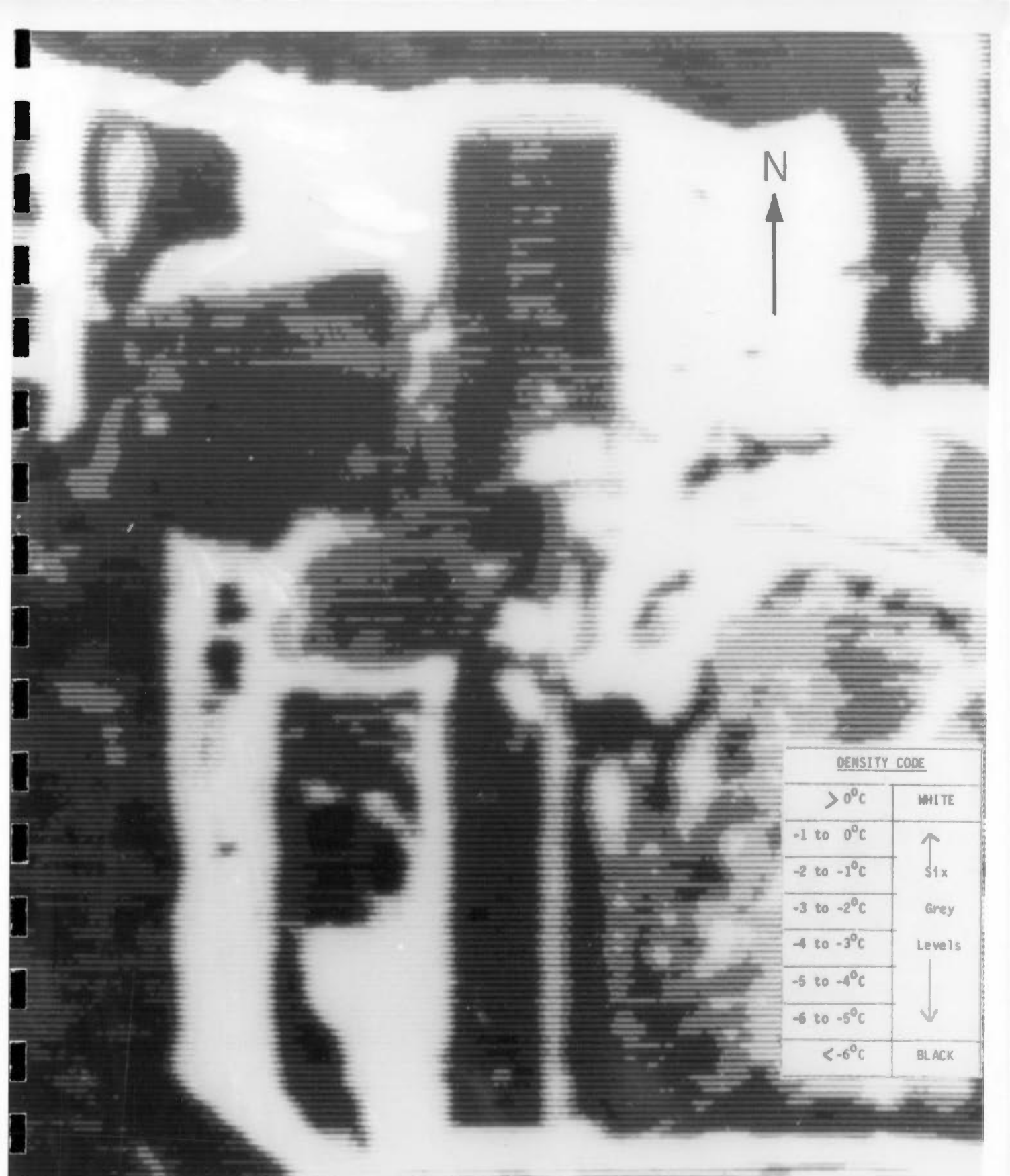
FIG. 4.6: Hollard College Royalty Centre, 11:10 P.M., March 26, 1978. Air temperature, -8.4°C. Wind, 10 kph approximately. Radiative sky temperature, -18°C. Thin overcast at 3.7km.
