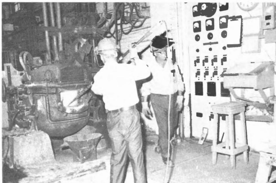
The temperature of a bath of molten alloy pipeline steel is being measured in a direct arc electric furnace in the experimental foundry.
