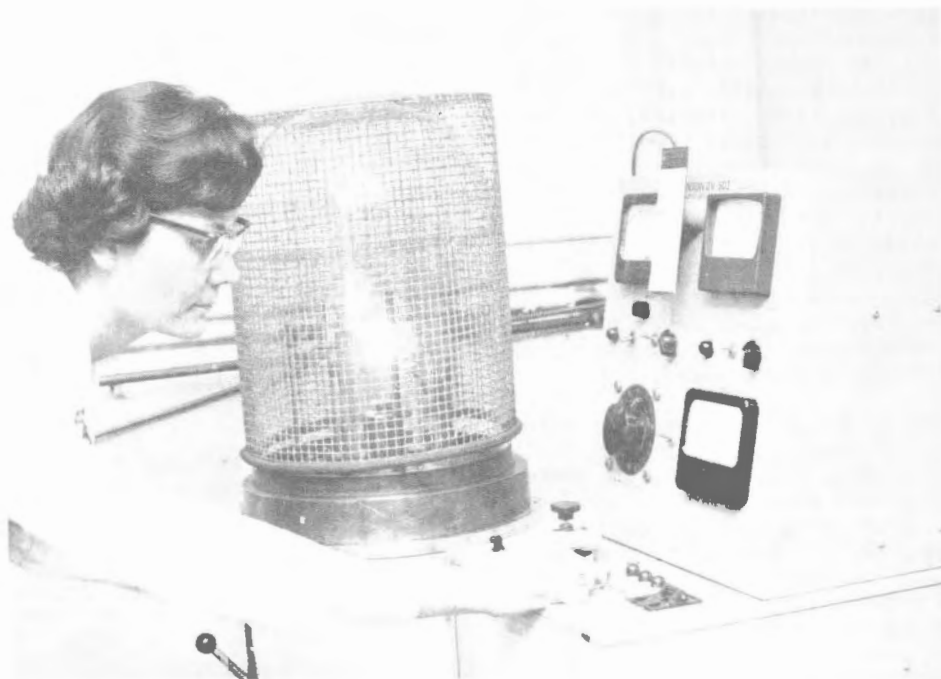
Specialized techniques are needed in the preparation of specimens prior to examination with an electron microscope. A carbon extraction replica of rail steel is being made here for examination at very high magnification.
