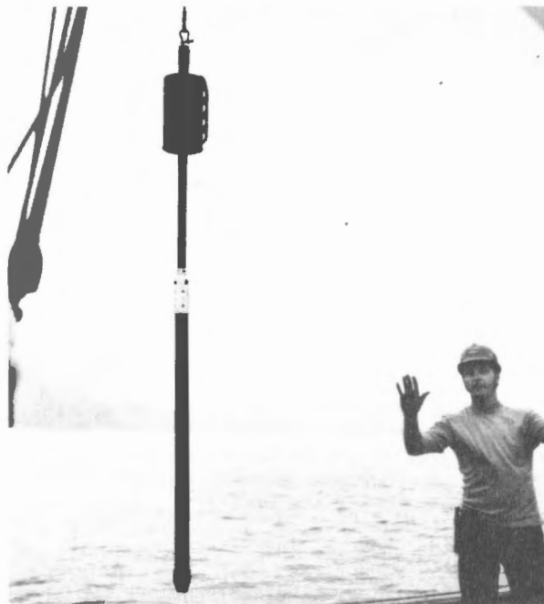
A Benthos gravity corer in use in the Straits of Canso by staff of the Atlantic Geoscience Centre.
