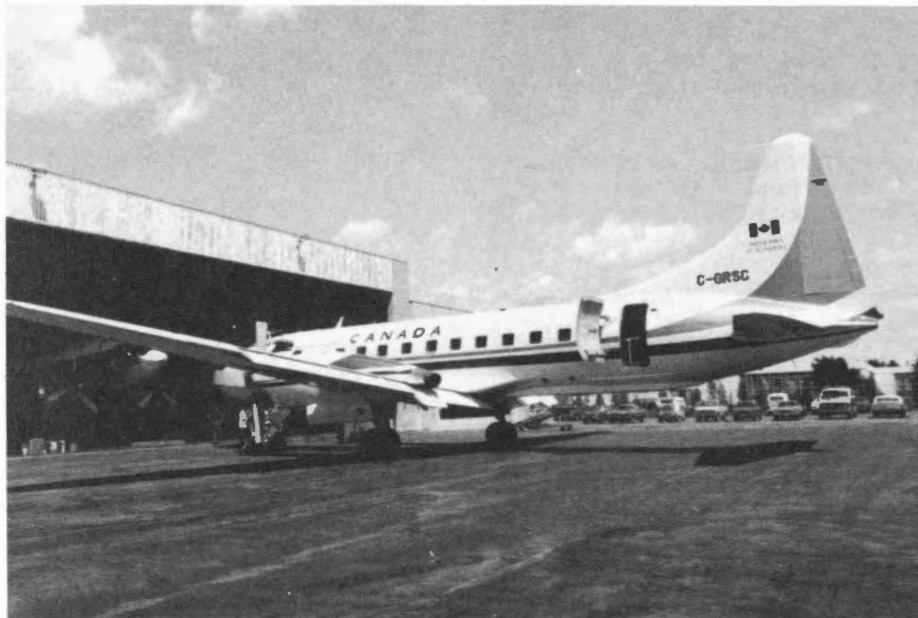
The Convair 580 aircraft is used for remote sensing investigations in the Arctic and offshore. It is now being used in an aerial hydrography project and is being outfitted with a synthetic aperture radar (SAR) for participation in the SURSAT project the objective of which is to determine how best to meet Canada's surveillance needs in the 1980's.
