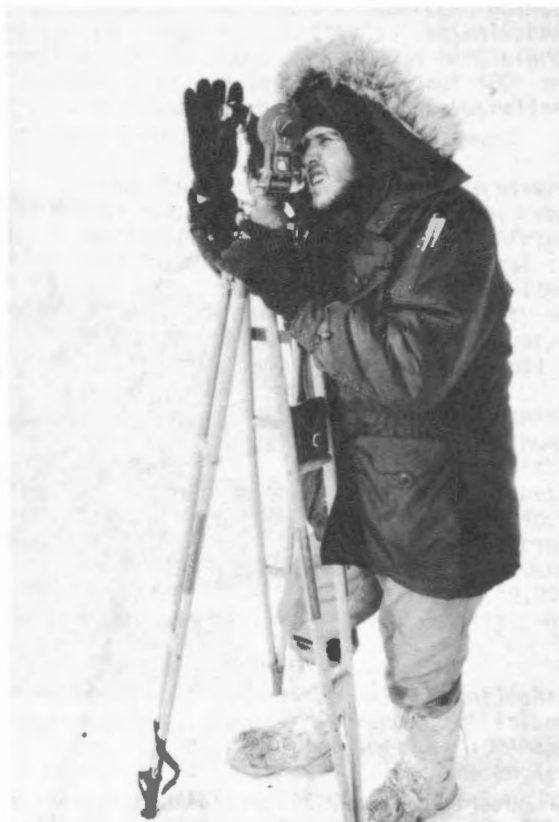
Under severe winter conditions a surveyor uses a theodolite to make observations.
