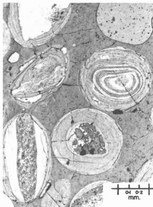
Photomicrograph of Peace River iron ore showing rounded oolites in ferruginous opal
