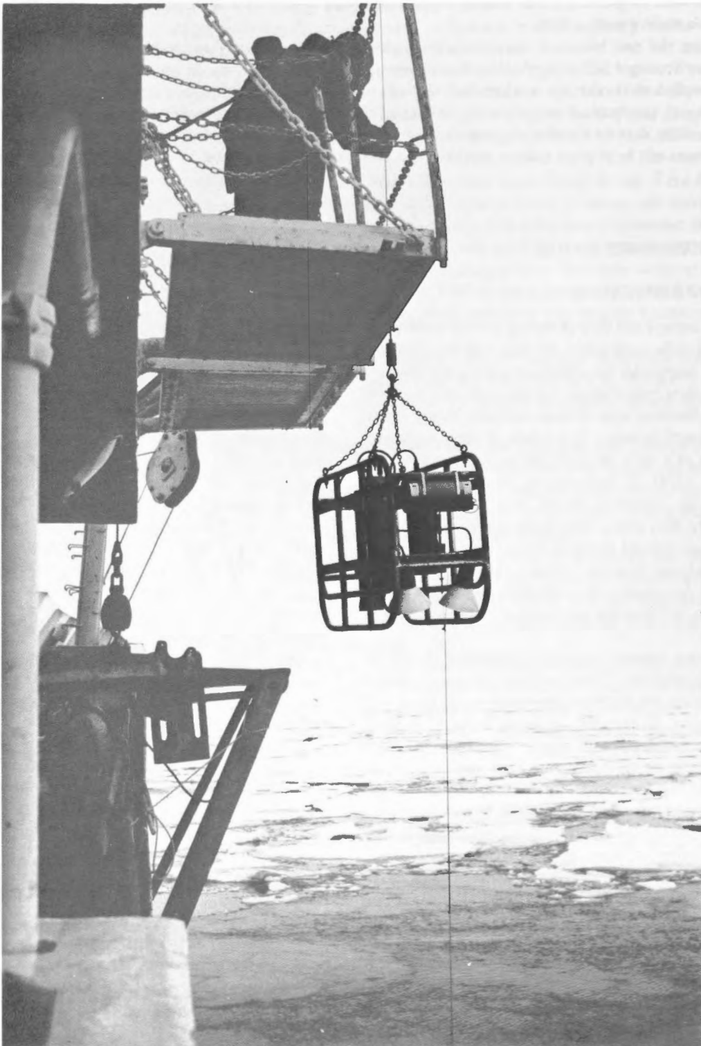
Umel underwater camera system being lowered in Lancaster Sound
