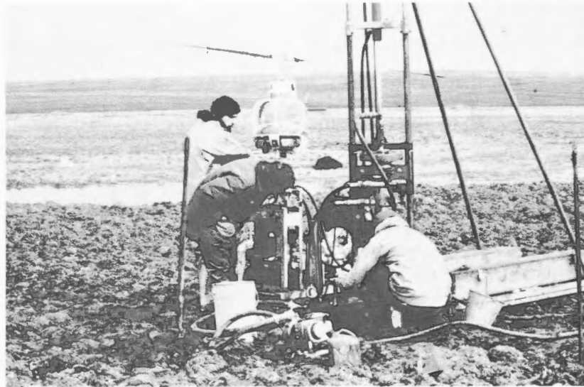
Soil sampling, Central Banks Island, N.W.T., using helicopter portable drill. GSC 202655-K
