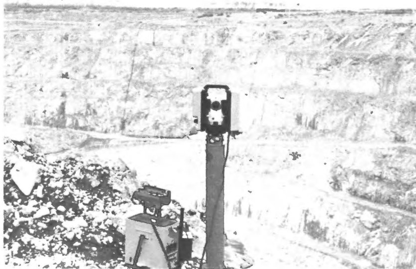
Laser theodolite in position to observe targets on opposite pit wall.
