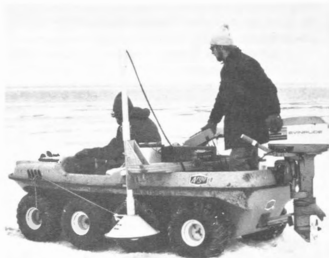
All-Terrain Vehicle equipped with echo sounding and sub-bottom profiling gear. The vehicle is capable of driving from a beach or an ice flow into open water. GSC 202653-N
