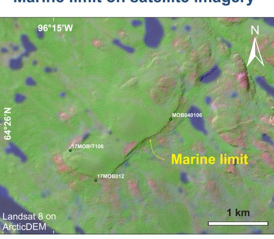
Trimline at 118 m elevation west of Baker Lake. Thick lacial sediments are found above the marine limit reworked sediments and bedrock outcrops occur below the limit of marine inundation.
