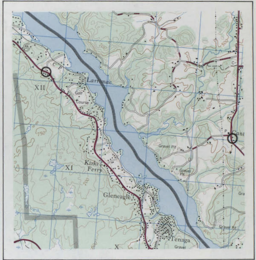
Figure 4. Part of the Wakefield, Quebec, Sheet, Scale 1:50,000, made from the air photo in Figure 5.
