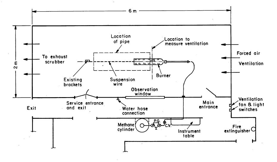
Fig. 1 - Layout of large scale gallery test for rigid plastic ducts.
