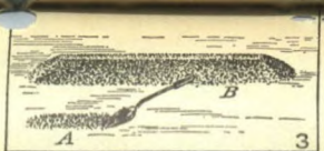
Mix by forming long pile. A—spreading out first shovelful. B—long pile completed
