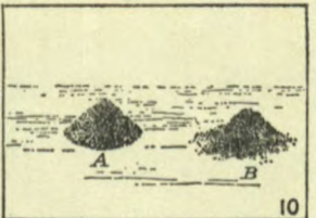
Long pile divided into two parts; A—reserve; B—reject
