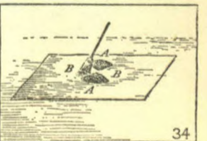
Fill two 5-pound sample containers from A, A, one for laboratory, one for reserve
