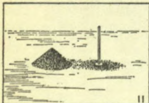
Crush 250-pound sample (fig. 10, A) to 1/2" size
