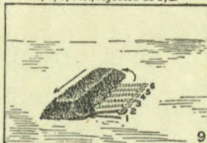
Halving by alternate shovel method. Shovelfuls 1, 3, 5, etc., reserved as 10, A; 2, 4, 6, etc., rejected as 10, B
