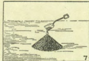
500 pounds crushed to 3/4" and coned
