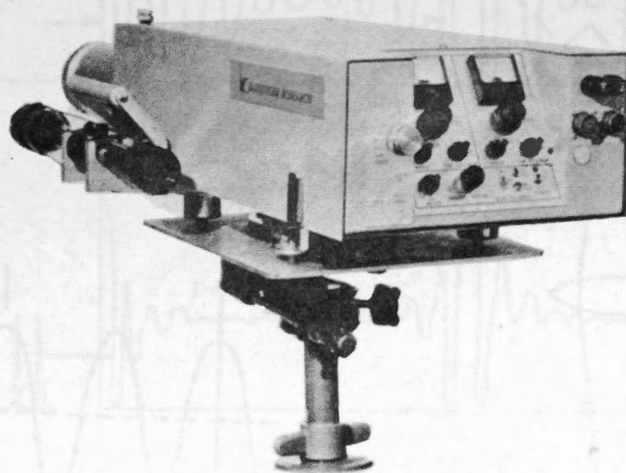
FIGURE 3 DUAL GAS CORRELATION SPECTROMETER COSPEC II
