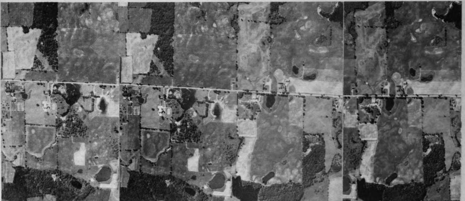
Figure 5. Hummocky morain landscape (Galt Morain). Stereotriplet. SAP, Hasselblad EL with Biotar 80mm, Panchromatic Tri-X film, Wratten 12, F-22, 1/500 sec. Flying height 8000 ft. above terrain, approx. scale of original 1:30.500, 12 August, 1971 h= 11,30 a.m.
