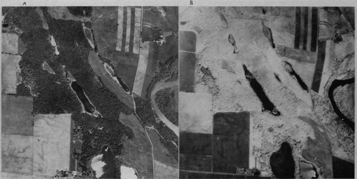
Figure 4. Pinehurst Morainic Ridge . Comparison of panchromatic and infrared photographs. SAP,Hasselblads EL, 15 July,1971,h=11,30 a.m., 1/500 sec.,Flying height 8000ft. a) Panchromatic, Tri-X film, Wratten 12, F-16½ b) Infrared Aerographic film, Wratten 87, F-5,6½
