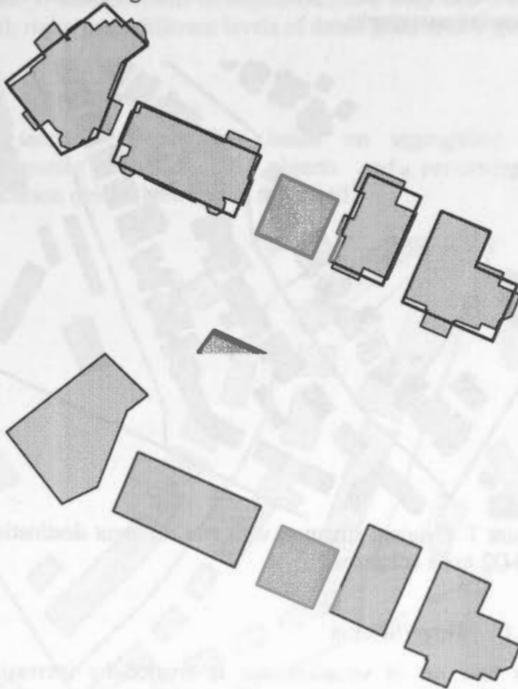
Figure 4: Simplification of object shape: a) overlay of simplified and original shapes, b) result of partial simplification: target shape without simplification.
