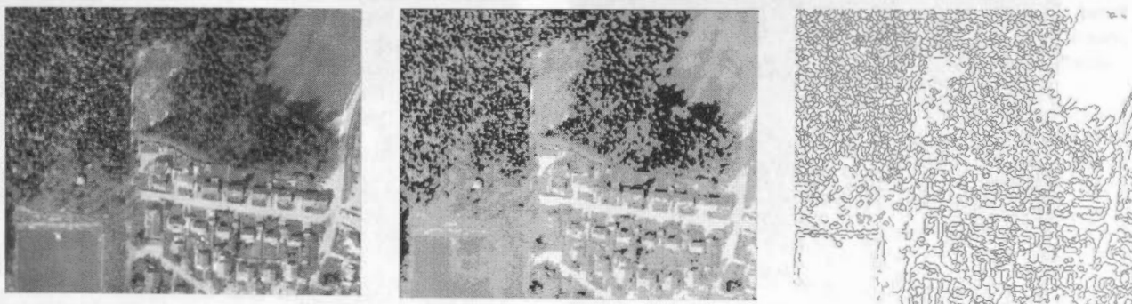
Figure 1. Given image (left) and exemplary point-based segmentation with four classes (middle), and contours as input for edge-based segmentation (right) - data courtesy of TopoSys GmbH -
