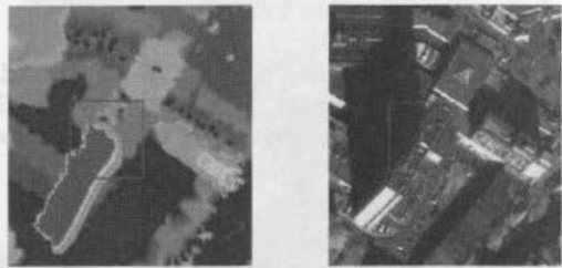
Figure 2. Planimetric shift due to local height relief
