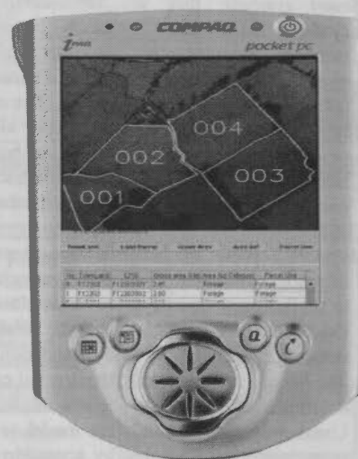
Figure 4. A LIMS application developed using e-Spatial™ technology and viewed on a PDA.
