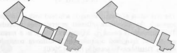
Figure 5: Aggregation of "irrelevant objects" – separation and visualization in full detail of destination object: a) overlay (outline), b) Result of aggregation.
