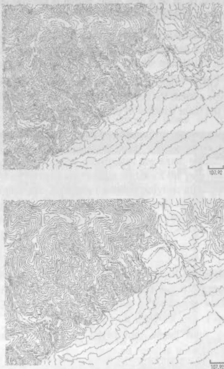
Figure 8. Simplified result. Upper image: original contour lines (1/2500: 44304 points / 1370 objects), lower image: simplified contour lines (1/10000: 21474 points / 1315 objects)
