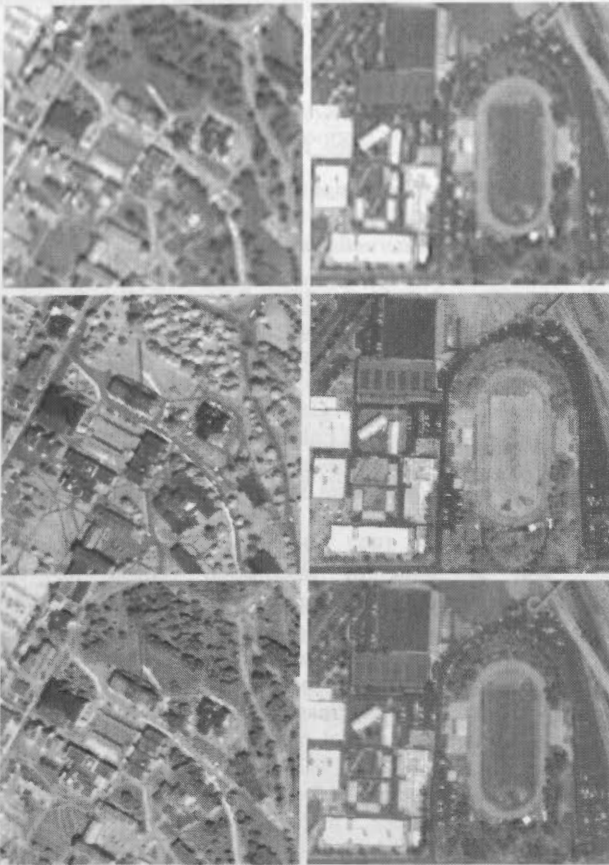
Figure 7. Minimized colour distortions of the new fusion technique. From top to bottom: original IKONOS natural colour images with 4 m resolution, original IKONOS panchromatic images with 1 m resolution, and IHS fusion results. Left: Fredericton, Canada. Right: San Diego, USA.
