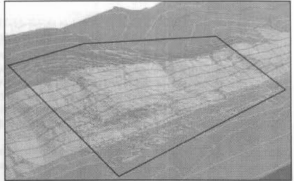
Figure 11. Merged GPS and photogrammetric derived DEMs (1 m contours)
