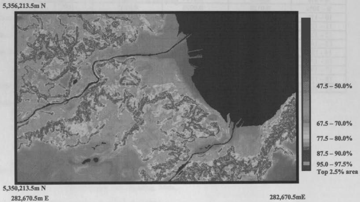
Figure 2. Landslide hazard prediction map based on 73 landslides (22 in 1967, 51 landslides in 1976 and 1996) and five layers (bedrock geology, forest coverage, elevation, aspect angle, slope angle maps) of geomorphological map information using likelihood ratio function model.
