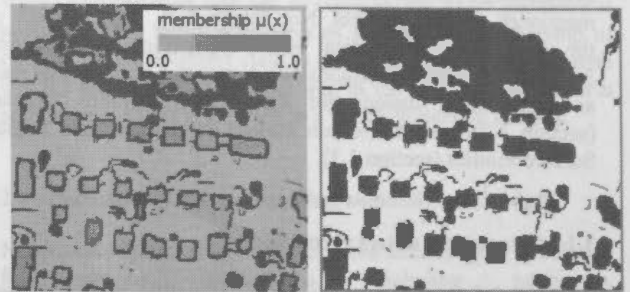
Figure 4. Intermediate results of terrain surface estimation: fuzzification based on "mean gradient" (left) and classification of non-terrain areas (in grey; right) - the test site is identical to that shown in figures 1 and 2
