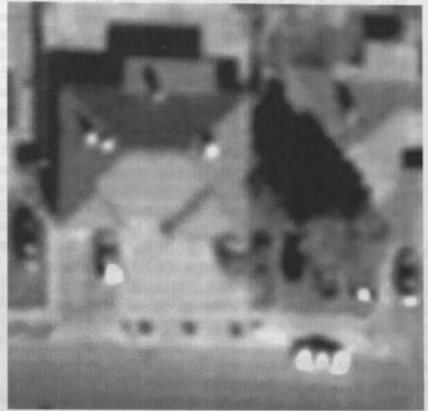
Figure 2: Partial resampling of Figure 1 using 16pt. \sin(x)/x kernel (400 x 400 pixels; 10-cm pixel spacing). Courtesy and copyright of DigitalGlobe, 2002
