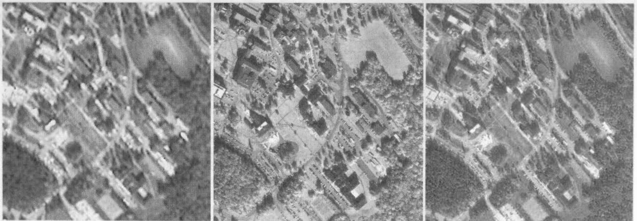
Figure 8. IKONOS images covering the University of New Brunswick, Canada before and after the fusion. Left: Original 4m natural colour image, Middle: Original 1m panchromatic image, Right: Automatically fused natural colour image of the new technique.
