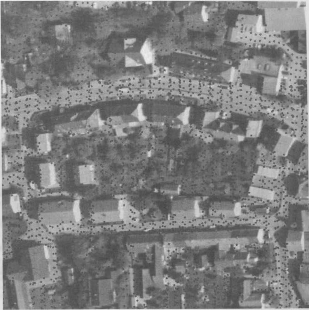
Figure 5. Digital orthophoto overlaid with LIDAR measurements
