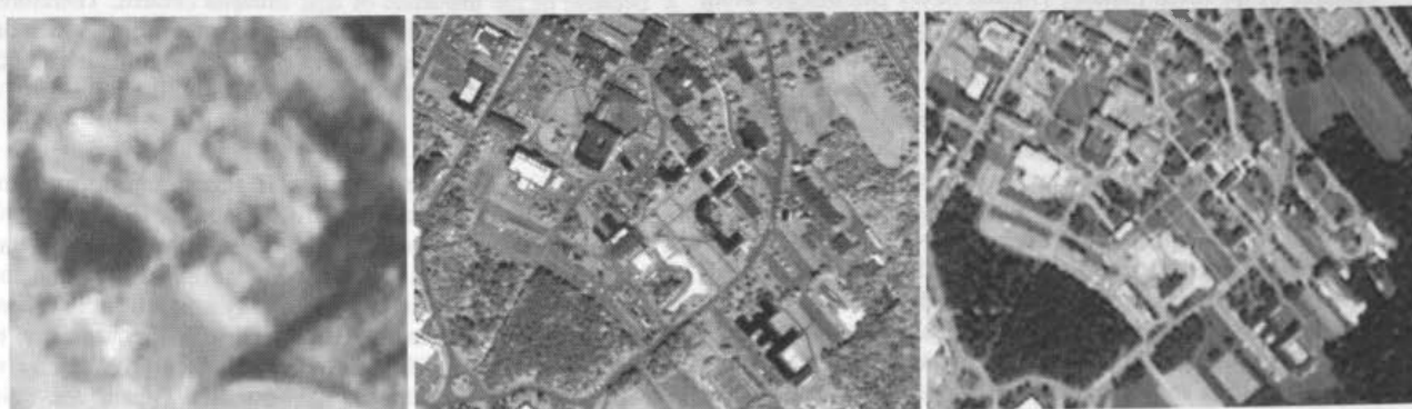
Figure 6. Comparison of grey value differences between SPOT panchromatic (left), IKONOS panchromatic (middle), and IKONOS Intensity (right) images (with a: left, b: middle, c: right)
