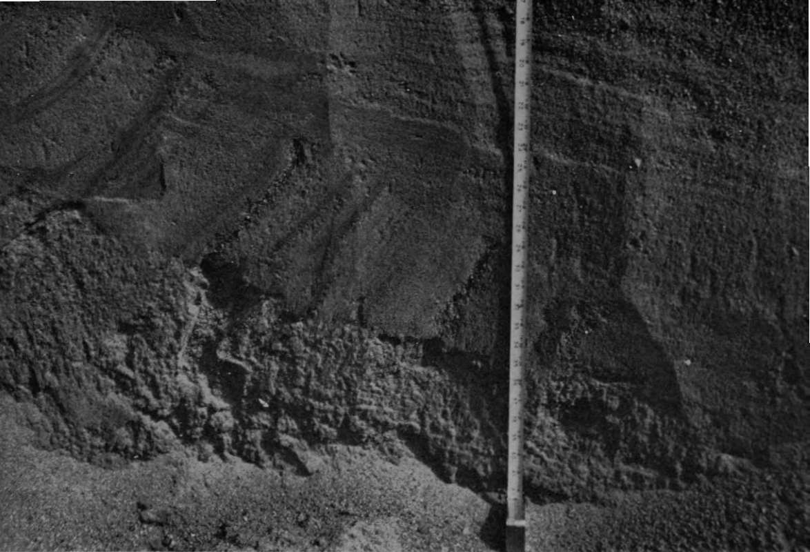
FIGURE 8. Photograph of a pit in RI showing the silt bands dipping steeply downglacier. The photograph should be compared with Figure 9, which is a sketch of the east wall of the pit.
