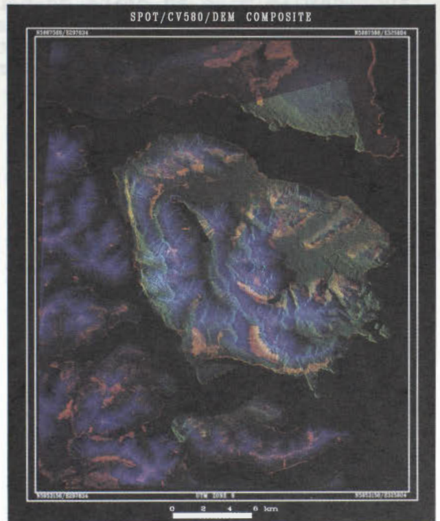
Figure 3d SPOT / C/X SAR / TRIM DEM Composite image; The SAR image (in green) does not perfectly overlay with the other data sets. For high relief areas, ortho-correction is required to correct for inherent SAR terrain distortions.
