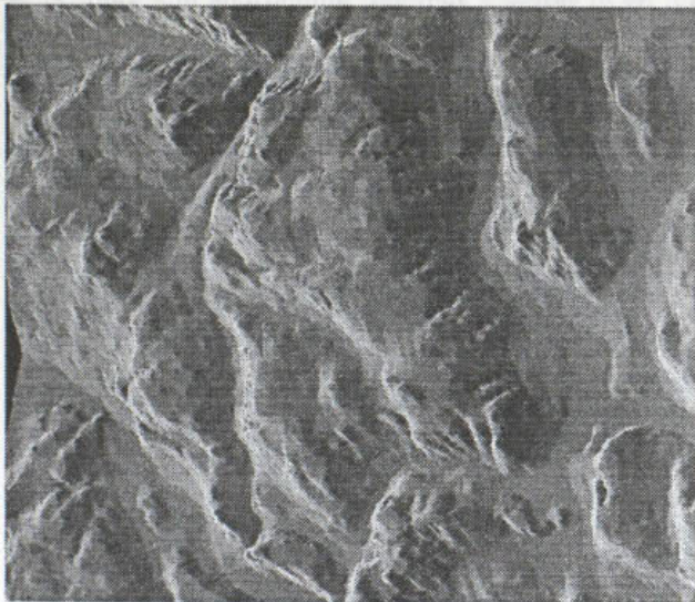
Figure 4: The simulated SAR image generated from the DTED shown in Fig. 3 and the known SAR platform parameters.
