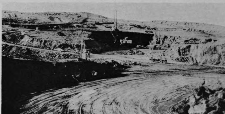
Figure 5. Detail of pit operations at Ferriman mine. Note the accumulations of large blocks of permafrost on the floors of the pits (centre and lower right), and the barren nature of the original land surface behind. September, 1957.
