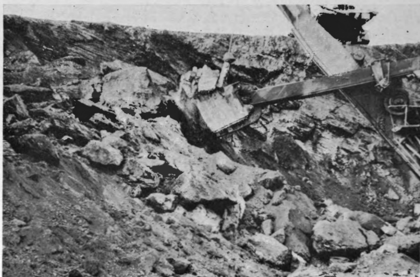
Figure 6. Detail of mining operations at Ferriman mine. Note the large boulders (permafrost) which are up to seven feet across. September, 1957.
