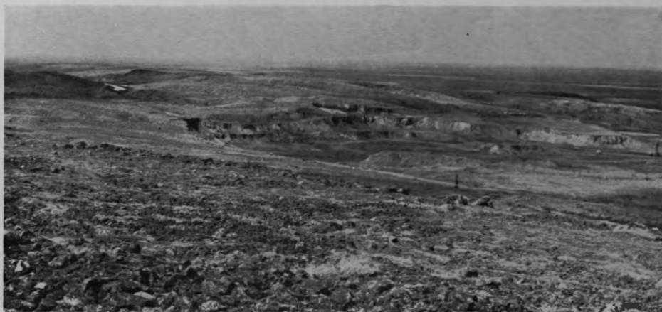
Figure 4. Ferriman mine, Schefferville, viewed from the high western ridge in the area of thermocouple installations. This orebody is predominantly in permafrost which in places exceeds 200 feet in thickness. Note the barren nature of the landscape. June, 1960.
