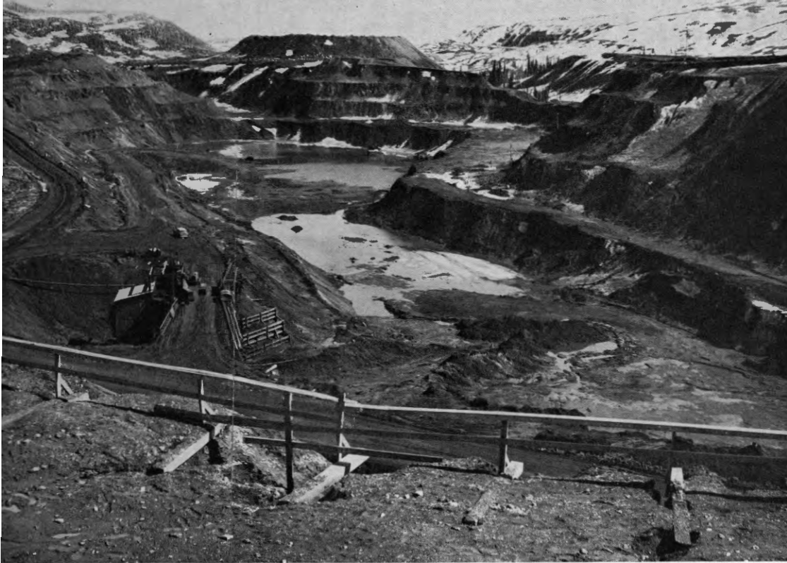
Figure 3. Ruth Lake mine, Schefferville. A panorama of one of the main ore-producing mines cut into unfrozen ore. Note the extensive nature of the excavation and the orderly development of the burms (mining levels). The screening plant is located in the bottom of the pit (left centre). May, 1960.
