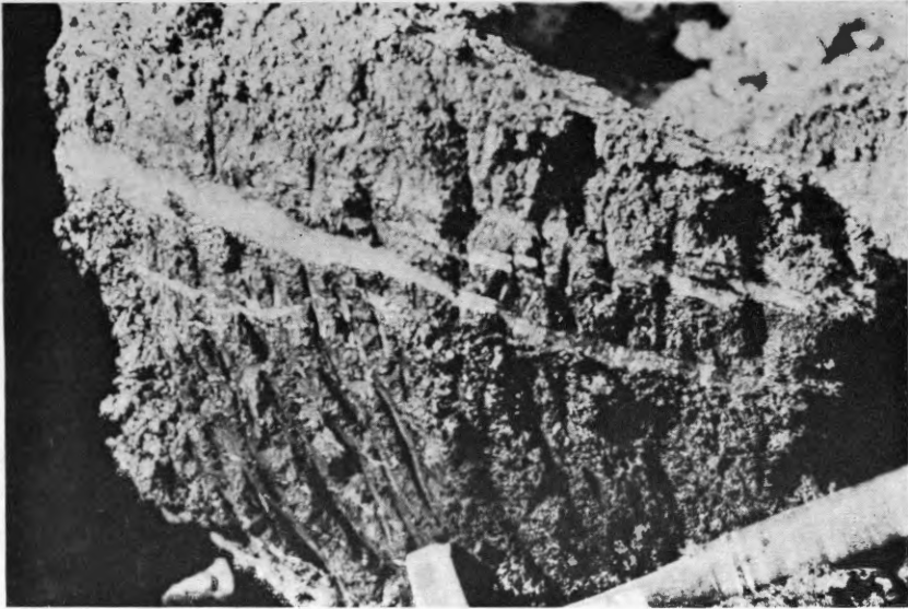
Figure 8. Lenses of ice can be observed frequently in the new sections resulting from a recent blast. The hammer provides the scale. June, 1960.
