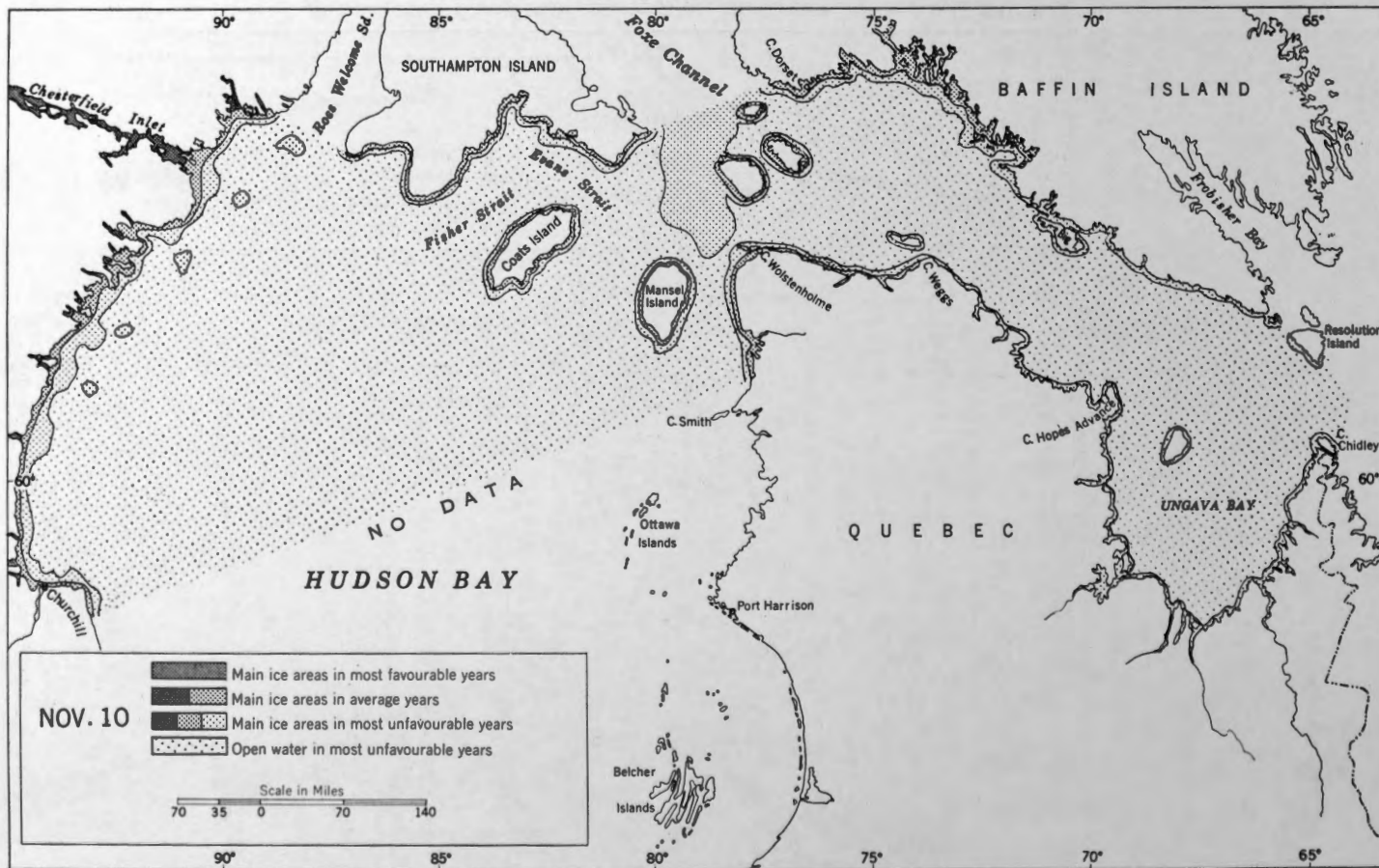
Figure 14. Limits of main ice areas along the Hudson Bay route on November 10.
