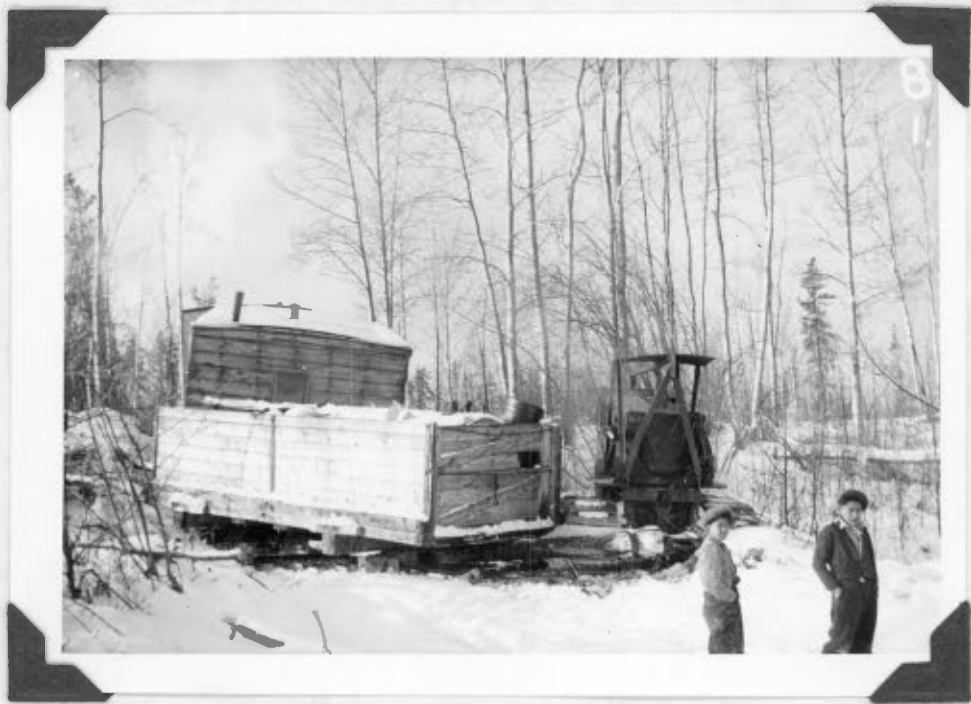
Mishap descending west bank of Hay River, showing jack-knifed train and broken bunting pole.
