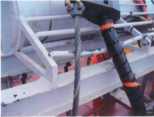
Bent in the steel bar at the top of the airgun sled.
