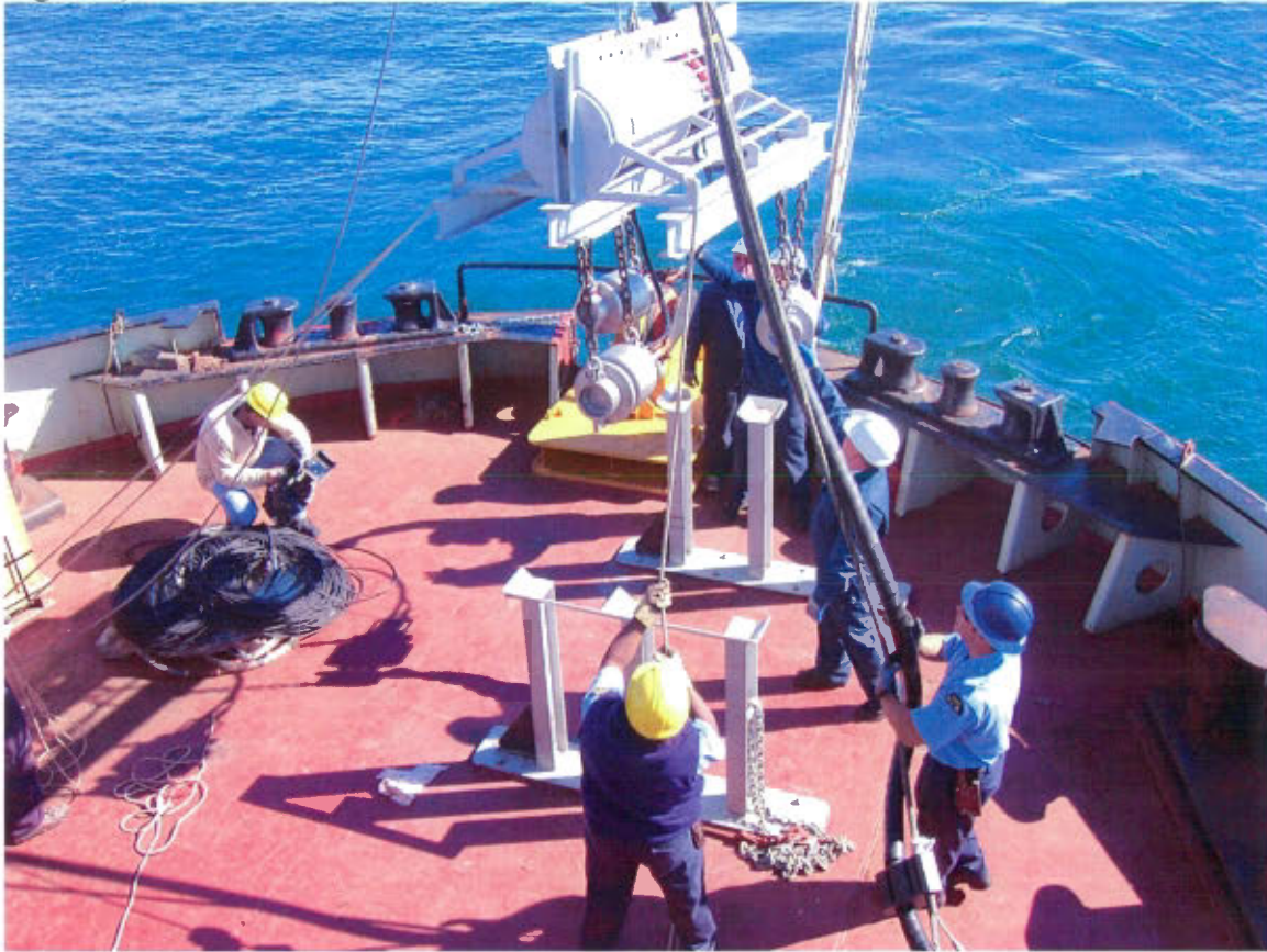
Figure 6: Tow Sled being lifted from the cradle
