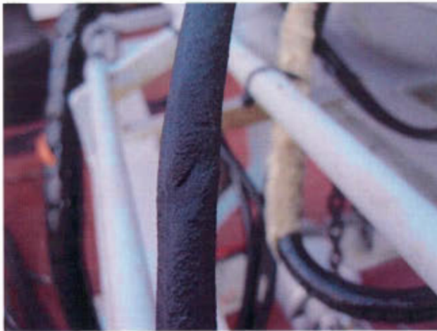
Puncture in the lead-in cable to the streamer.
