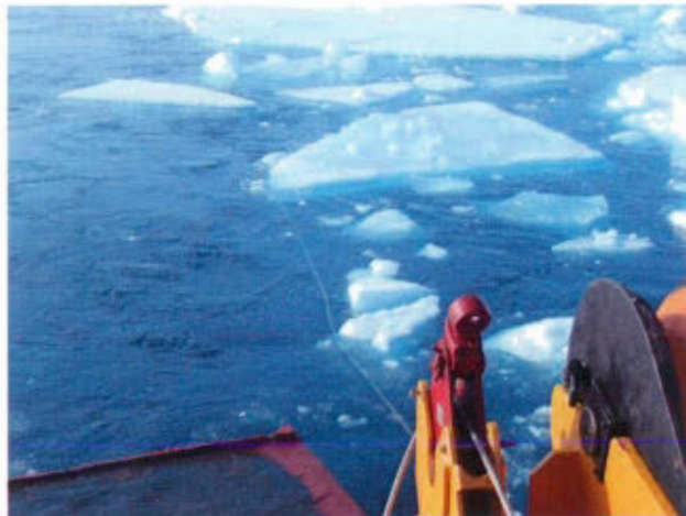
The streamer is swimming at the surface until the airgun array is lowered into the water.
