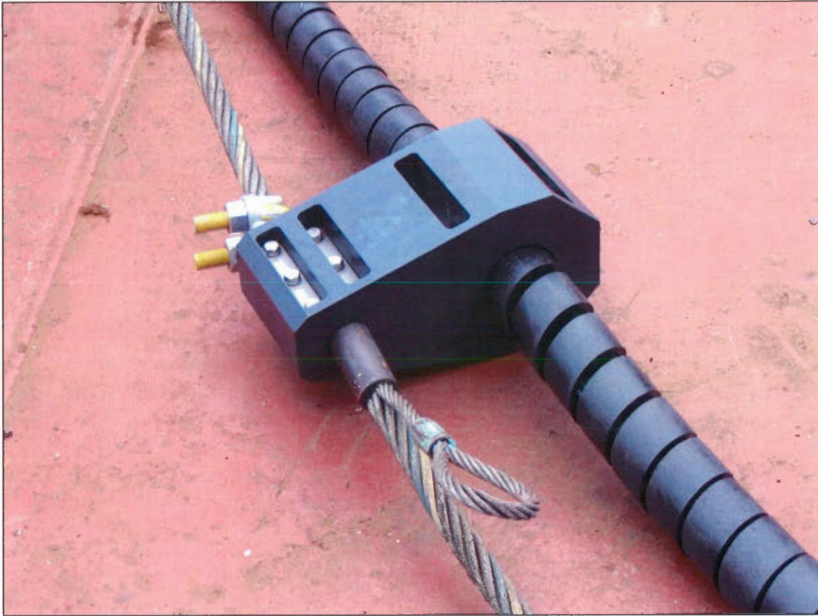
Figure 2: Bundle Clamp affixed to Tow Sled Pull Cable Showing “break out eye”
