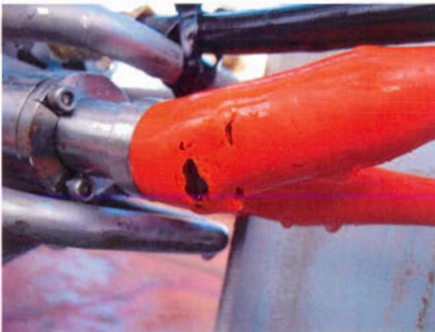
Dented electric connector at the starboard airgun.
