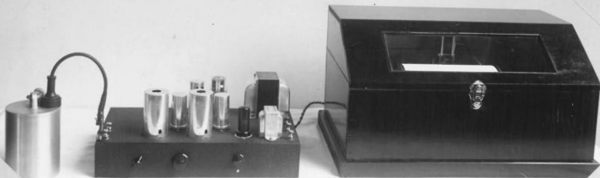
Fig. 8. Assembly with Heiland Geophone Pick-up
