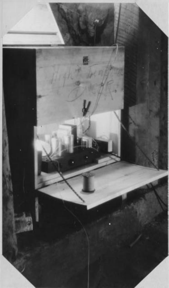
Fig. 9. Crystal Detector Set-up on the 2950-foot Level
