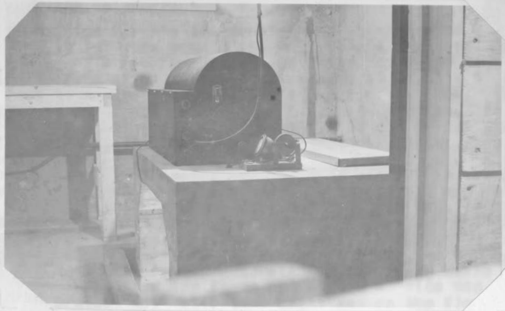
Figure 11. Camera on Pier at Kirkland Lake
