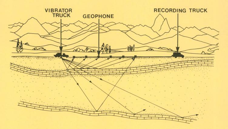
which they pulse, the data produced by seismic surveys permit the production of a threedimensional model of the depths of the earth.
