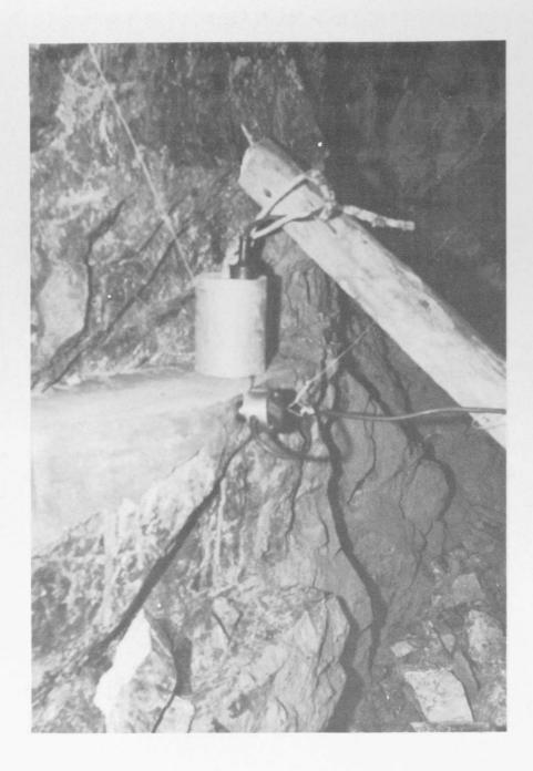
Fig. 21 Heiland Geophone and Crystal Detector (3950-ft. Level).
