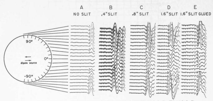
Figure 6. Shear waves from a dipole source (A) No slit; (B) 0.4 inch slit; (C) 0.8 inch slit; (D) 1.6 inch slit; (E) 1.6 inch slit glued. Downward trace motion corresponds to counterclockwise rotational motion on the model.
