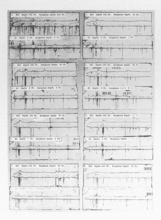
Fig. 50 Comparison of Recording in Adjacent Deep and Shallow Holes (deeper records).
