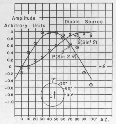
Figure 7. Observed and theoretical amplitude variation with azimuth for a dipole source.
