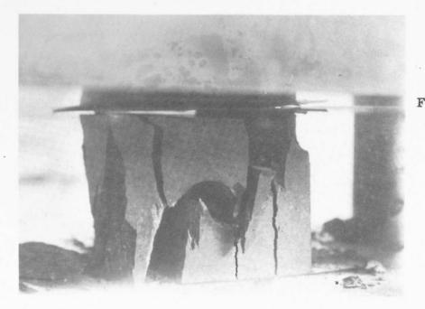
Fig. 37 Small Syenite Block after Crushing.
