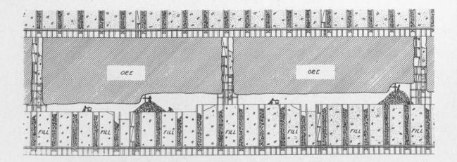
Fig. 15 Horizontal Cut-and-fill, Open Stope
