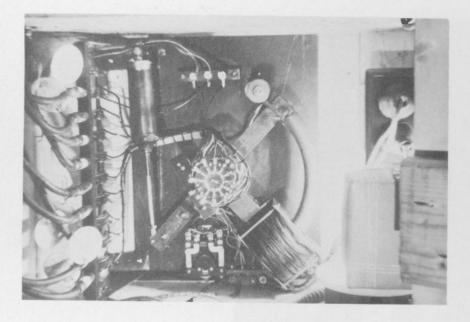
Fig. 71 Magnetic Stepping Switch.
