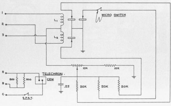
MICROSEISMIC RECORDER - U.S. BURERU OF MINES.
