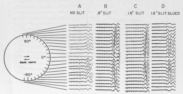
Figure 5. Compressional waves from a dipole source. (A) No slit; (B) 0.8 inch slit; (C) 1.6 inch slit; (D) 1.6 inch slit glued. Upward trace motion corresponds to outward motion on the model.
