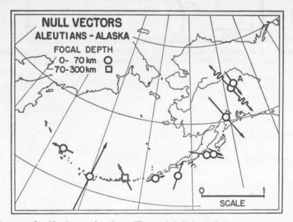
Figure 8. Null vectors for Aleutian earthquakes. The symbol designated A represents a solution by ADKINS (1940). In this, and in subsequent diagrams, null vectors of greater than unit length have been indicated by a compressed arrow.
