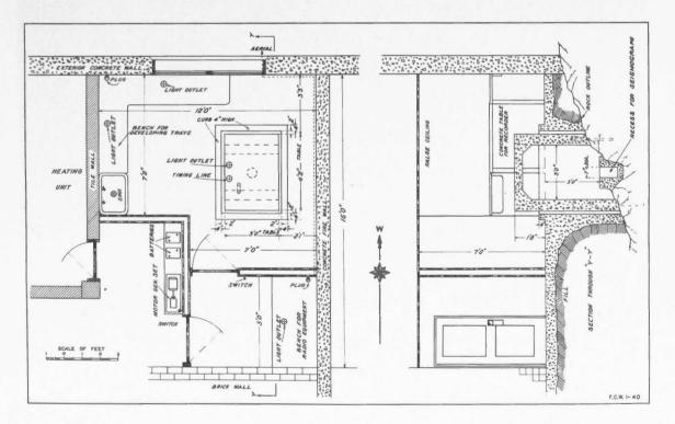
Fig. 6 Surface Seismograph Recording and Developing Room.
