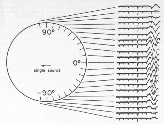
Figure 2. Compressional waves from a singlet source. Upward trace motion corresponds to inward motion on the model.
