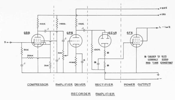
Fig. 83 Wiring Diagram: Recorder Amplifier, Obert Recorder.
