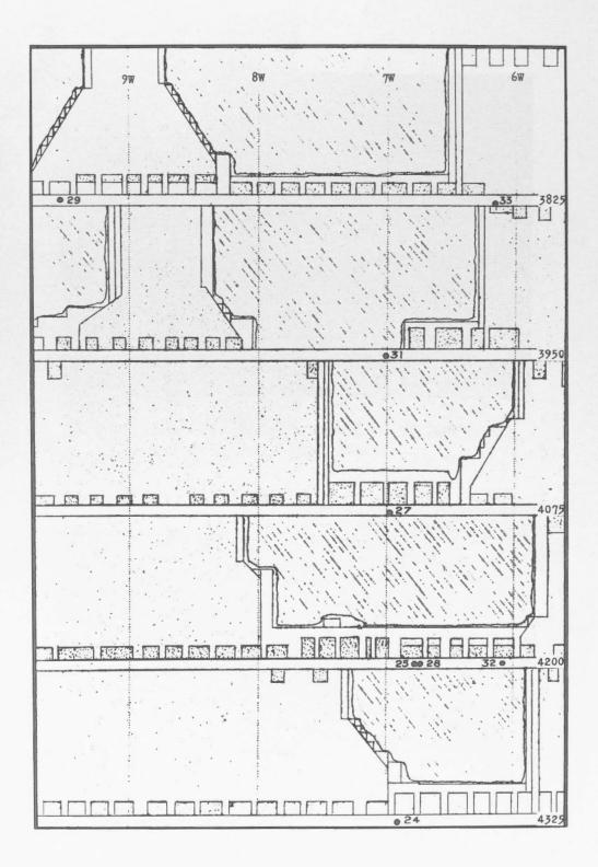
Fig. 58 Sections of West Pillar Affected by Rockburst of January 29, 1943.
