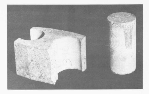
Fig. 87 X-shaped Specimen (Test 21; BM-390) and 2D Specimen
