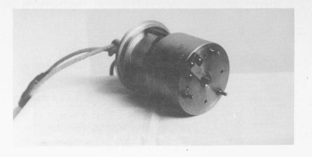
Fig. 18 Interior Heiland Geophone, Mine Seismograph.
