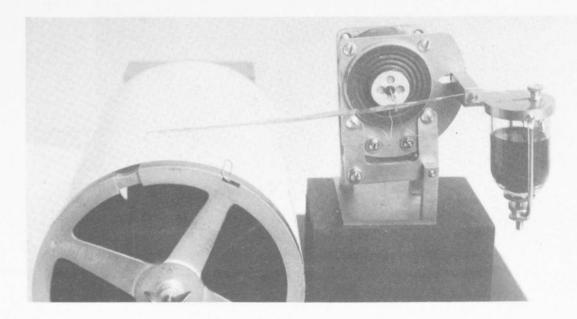
Fig. 20 Hollinsworth Recorder (pen detail).
