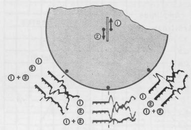
Figure 8. Elementary and composite compressional pulses from a dipole-fault model. Upward trace motion corresponds to inward motion on the model.
