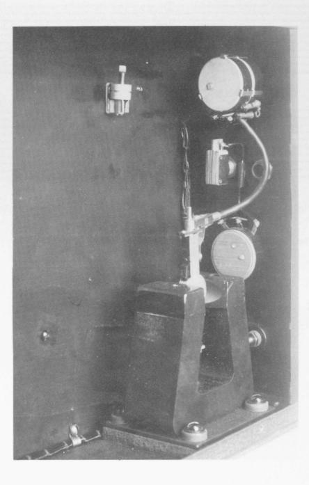
Fig. 4 Galvanometer Assembly, Surface Seismograph.
