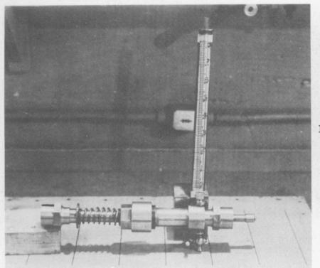
Fig. 22 Hydraulic Strain Gauge
