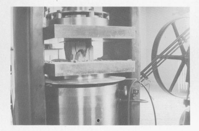
Fig. 36 Rock Crushing Experiments with Hollinsworth Gauge.
