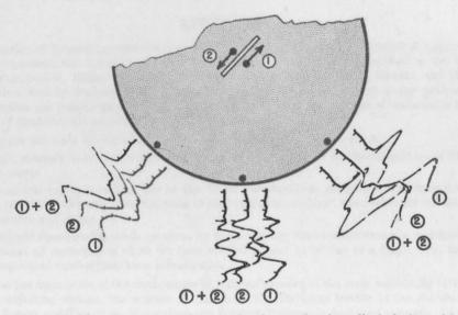
Figure 10. Seismograms showing elementary and composite shear pulses in a dipole-fault model. When reading seismograms from left to right, upward trace motion corresponds to counterclockwise rotational motion on model.
