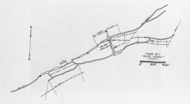
Fig. 8 Plan of 3075-ft. Level, Lake Shore Mines.
