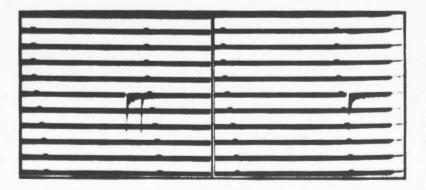
Fig. 41 Bursts I, I<sub>a</sub> and J as Recorded on the Lake Shore Surface Seismograph, July 30, 1941.
