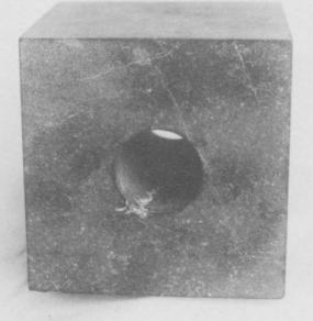
Fig. 38 Porphyry Specimen  $\underline{P}$  after Pressure to  $\overline{9}$ , 150 lbs/sq. in.
