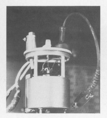
Fig. 43. Heiland Geophone with Sensitivity Tester.
