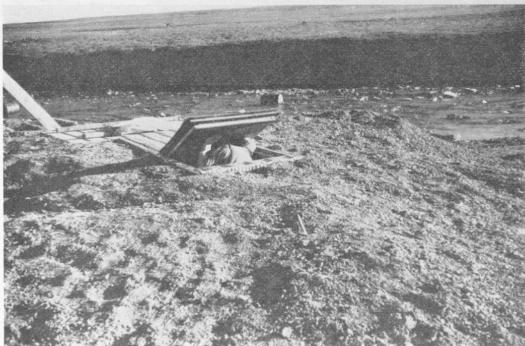
FIGURE 4—The seismometer shelter buried with gravel. The trapdoor leads to the stairway mentioned in the caption of FIGURE 3.
