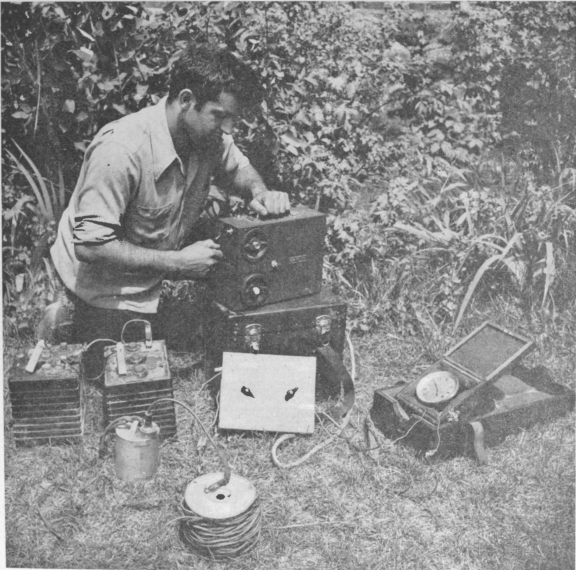
FIGURE 1—The blast timing equipment. It consisted of a six-channel seismic prospecting camera with storage batteries to supply power, a geophone and reel of cable of suitable length, a chronometer to indicate seconds and a control panel to adjust time mark amplitude.
