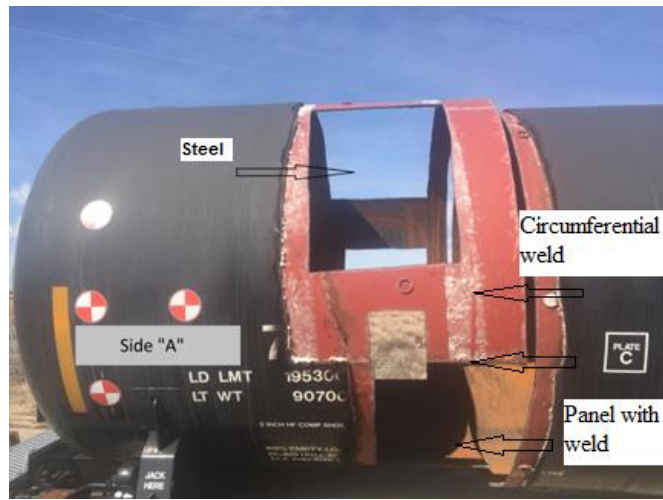
Figure 1. US Federal Railroad Administration impact-tested tank car, showing location of TC128B panel used in this work. Photo provided by Nolan Hanson of the Transportation Technology Center, Inc.
