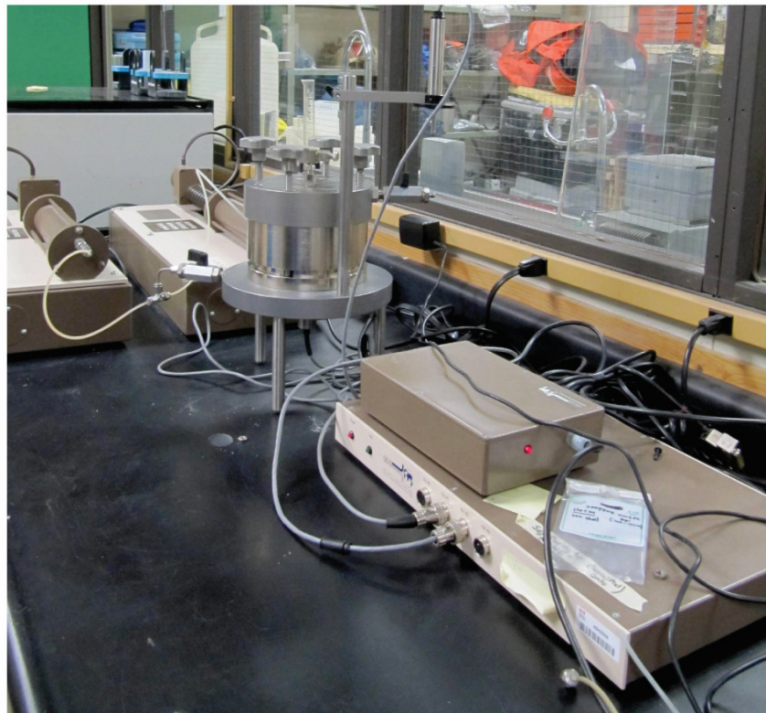
Figure 15. Rowe cell consolidation testing system. Photo by K. MacKillop, NRCan photo 2021-708.
