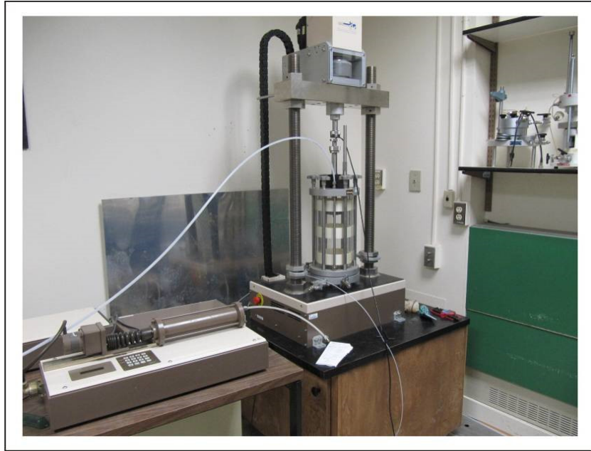
Figure 13. The GDS electromechanical dynamic triaxial loading system. Photo by K. MacKillop, NRCan photo 2021-706.
