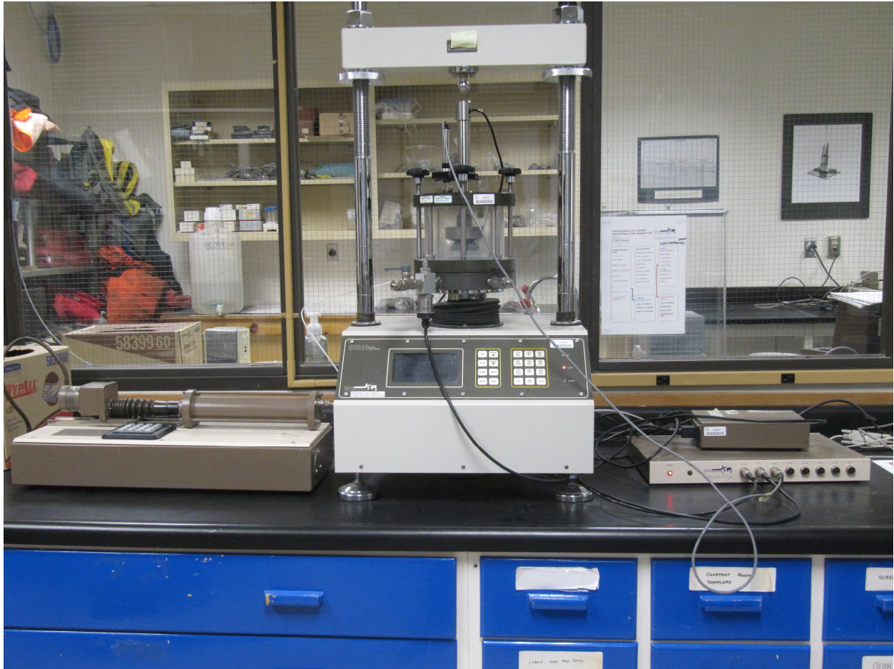
Figure 16. CRS cell consolidation system. Photo by K. MacKillop, NRCan photo 2021-520.
