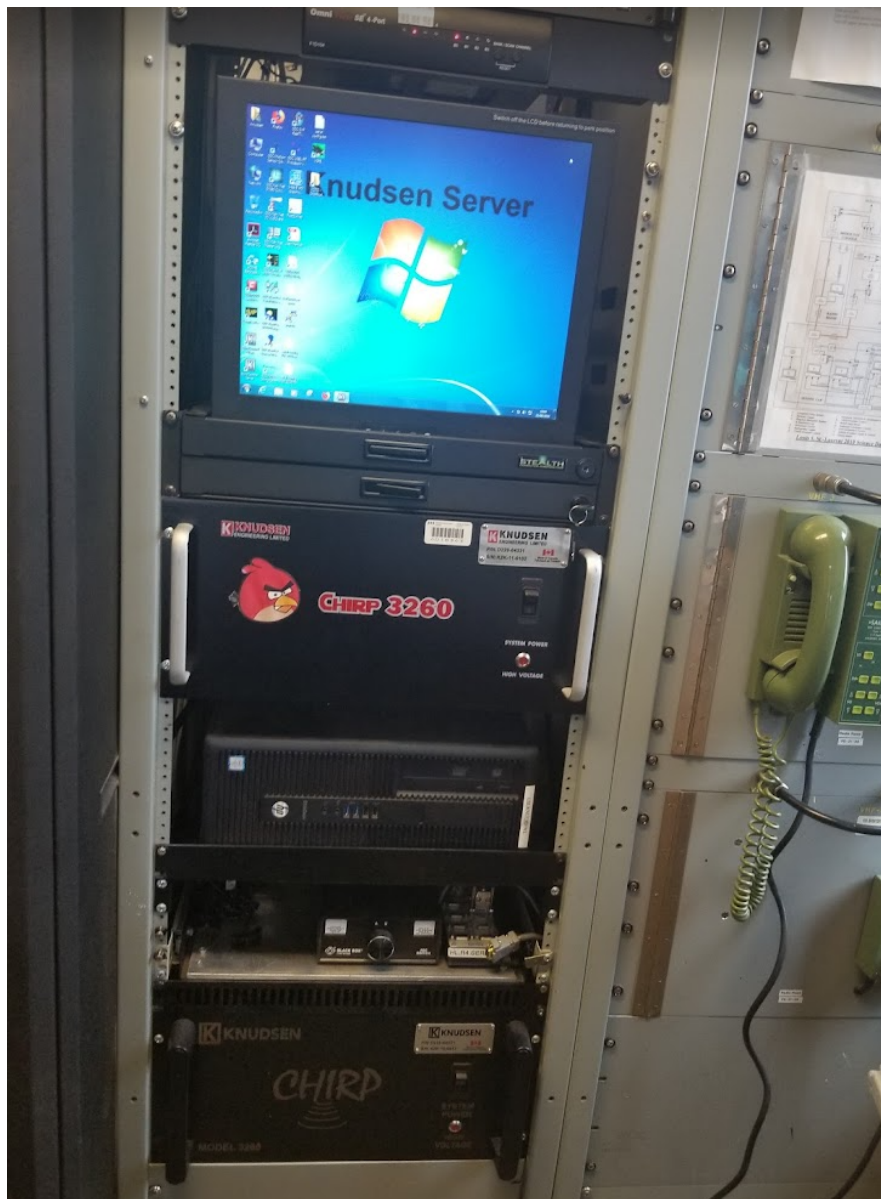
Figure 3. Knudsen 3.5 kHz sub bottom profiler server. Photograph by V. Kostylev NRCAN photo 2021-503.
