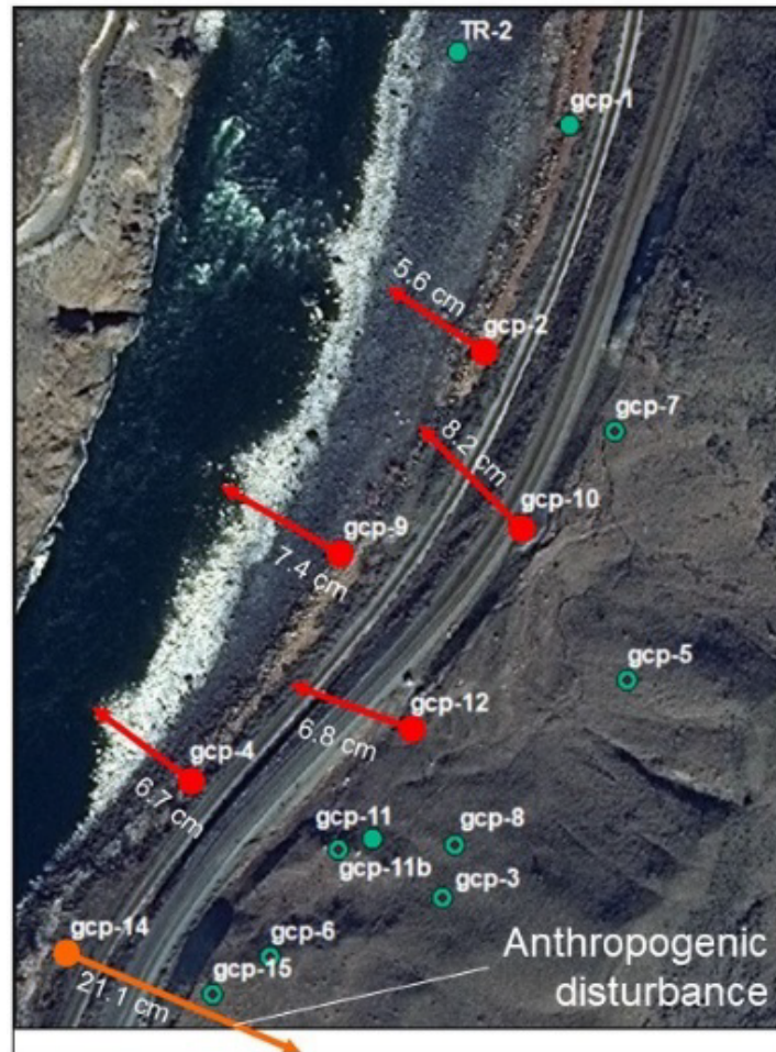
Figure 12 RTK-GNSS change detection of ground control points (GCPs) across Ripley Landslide from September 2019 to September 2020.
