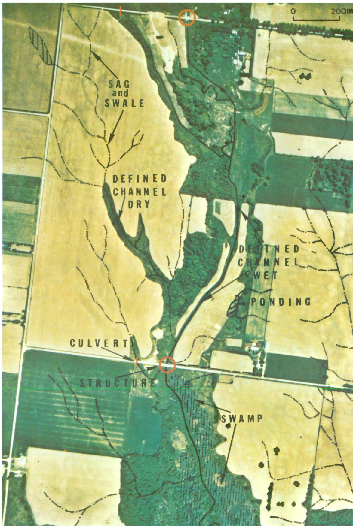
Figure 2 Surface Drainage Parameter, showing the level of drainage details required for the Environmental Surveillance Project.
