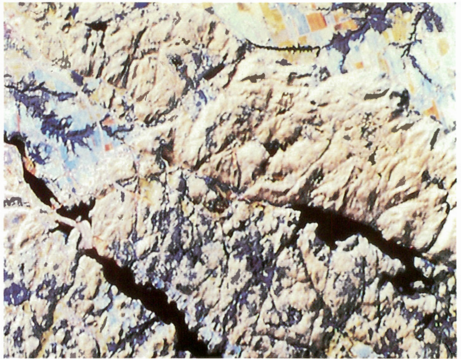
Enhancement of MSS bands 4, 5 and 7 over the Gatineau Hills, Quebec. Structural patterns related to faults and fractures in the Shield rocks are apparent in comparison with the flat agricultural lands of the St. Lawrence Lowlands.
